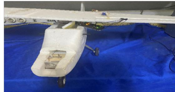
**Fig. 6:** Hardware setup for actuation system
