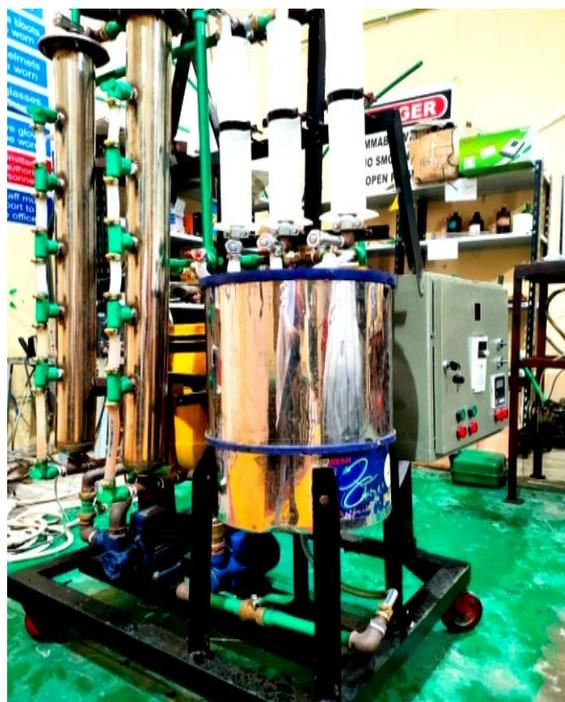
Figure 5, b: Photographic view of machine biodiesel production.
