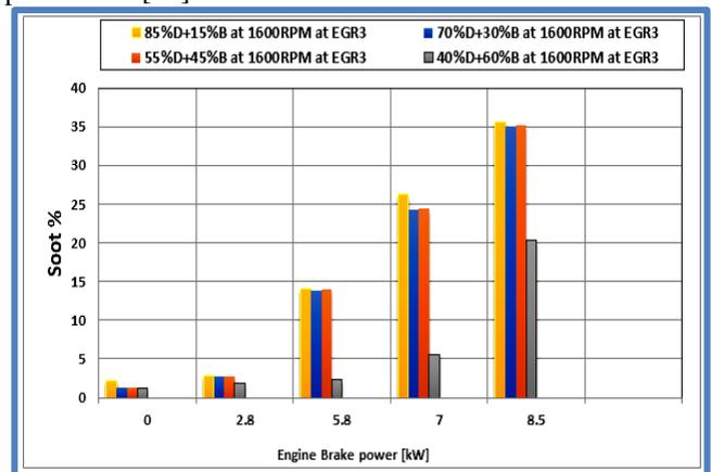
Figure 14. Illustrates the density of the soot (smoke) blends at engine brake power (loads) with EGR.
