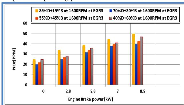
Figure 13. the nitrogen oxide (NO<sub>x</sub>) blends at various engine brake power levels (loads) with EGR.
