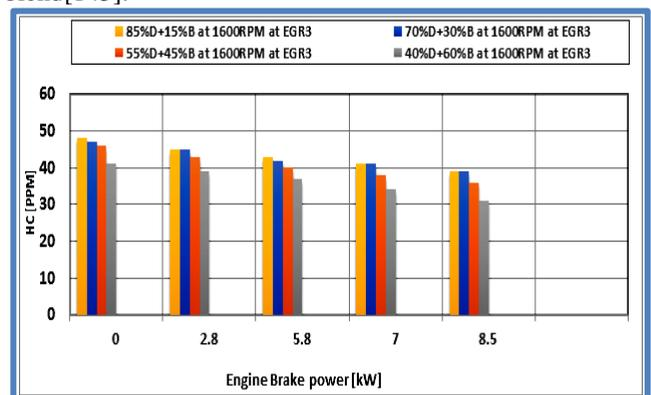
Figure 10. The emissions of total unburned hydrocarbons (HC) blends at various engine brake power levels (loads) with EGR.
