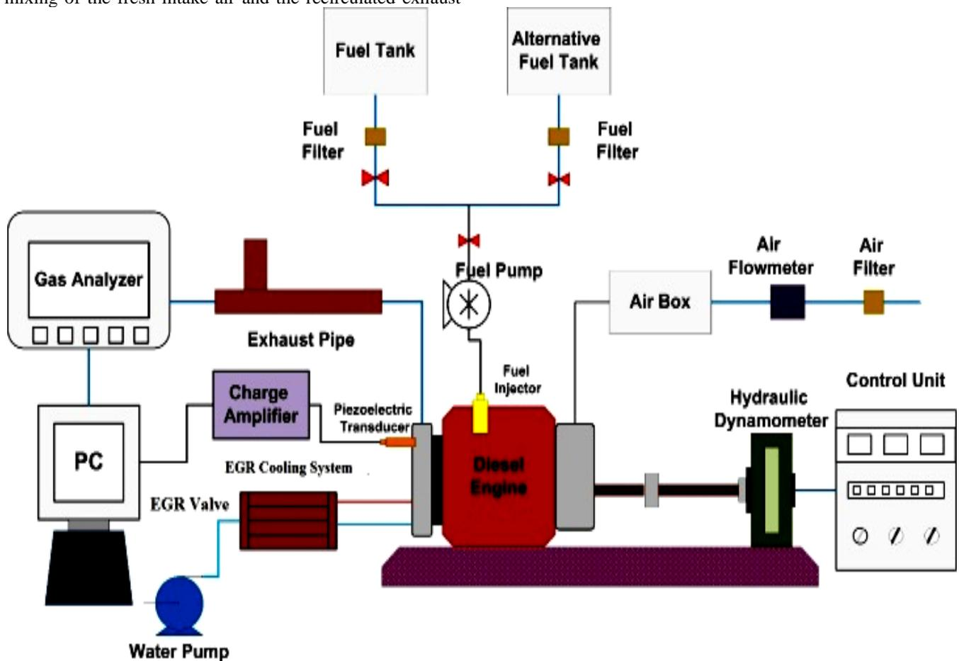
Figure 1. Schematic the operating machine diagram
