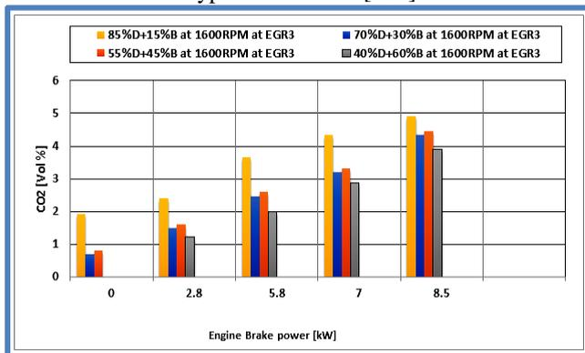
Figure 11. The emissions of carbon dioxide (CO<sub>2</sub>) blends at various engine brake power levels (loads) with EGR.
