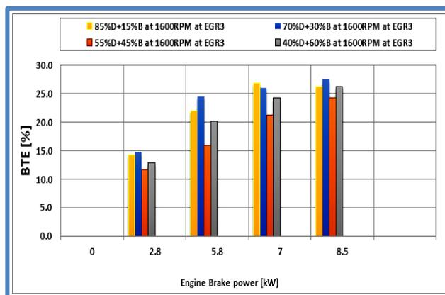
Figure 8. Change in brake thermal efficiency (BTE) blends at various engine brake power levels (loads) with EGR.
