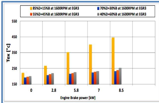
Figure 9. Changes in Exhaust Gas Temperature at various engine brake power levels (loads) with EGR.
