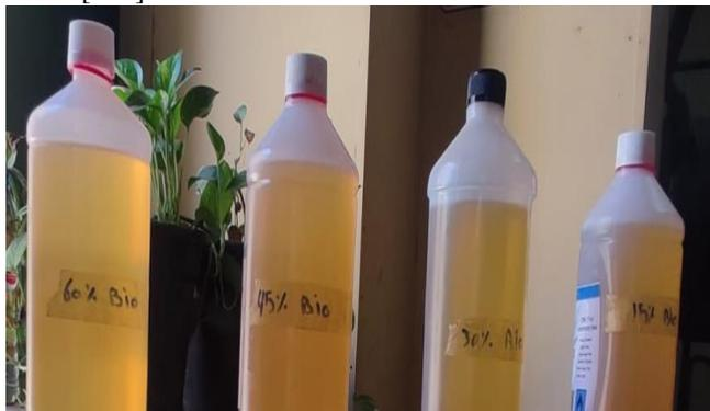
Figure 6. Four biodiesel/diesel blends
