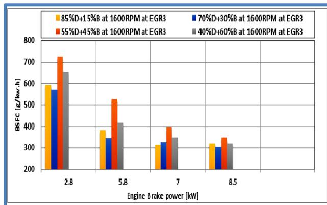
Figure 7. Illustrates the brake specific fuel consumption (b.s.f.c) blends at various engine brake power levels (loads) with EGR.
