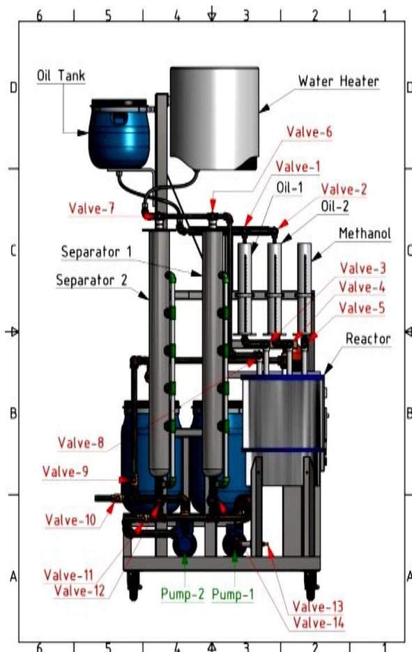
Figure 5, a: Schematic the operating machine diagram.
