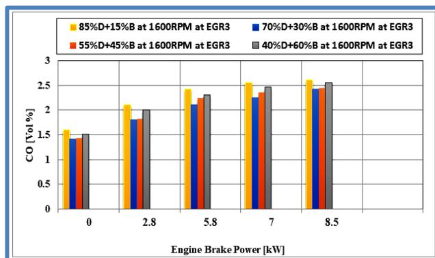
Figure 12. illustrates the carbon monoxide (CO) emissions blends at various engine brake power levels (loads) with EGR.
