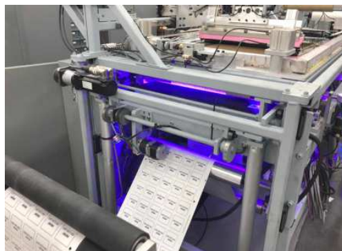
Figure 1. UV LED ink-curing printing technology (Packaging Strategies, 2021)
