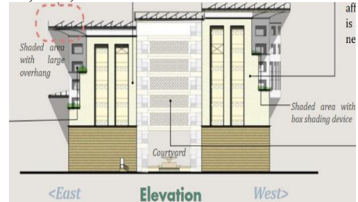
Figure 8: large overhang roof in West and East elevation.
