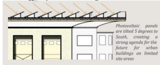
Figure 11: Photovoltaic panels are tilted 5 degrees to South. Source: ((DPAP), 2022)
