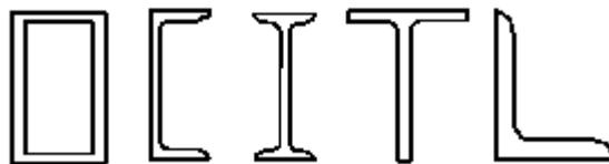
**Fig. 3: Capping Beam Shapes**
