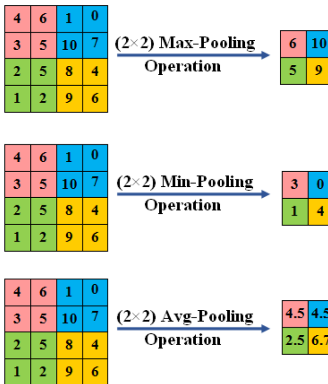
Figure 13. Examples of Different (2 \times 2) Pooling Operations of CNNs.
