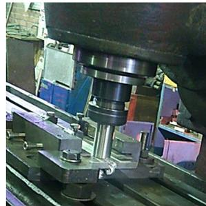
**Fig. 3 FSW Configuration.**
