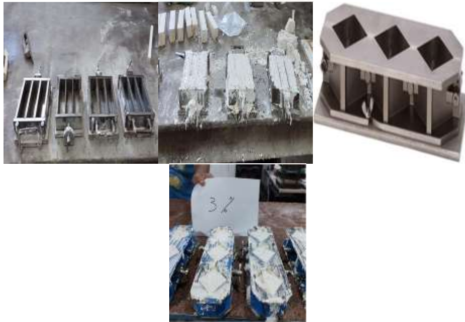
Fig.3. Molds used for casting samples
