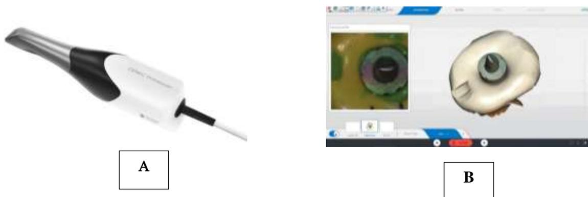
**Figure (2):** (A) Primescan Intraoral scanner, (B) Scanned metal die
