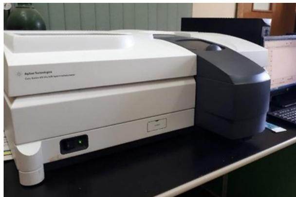
**Figure (6):** Agilent Cary 5000 spectrophotometer
