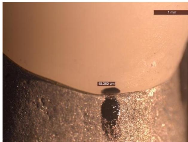
**Figure (5):** Margin adaptation of pilot crown under 30X magnification
