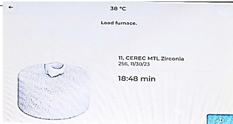
**Figure (4):** Sintering time for CEREC MTL Zirconia crown as shown on CEREC SpeedFire’s screen.
