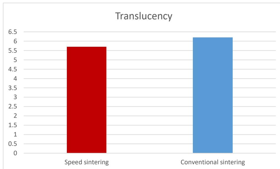
**Figure (7):** Bar chart showing translucency between speed sintering and conventional sintering.
