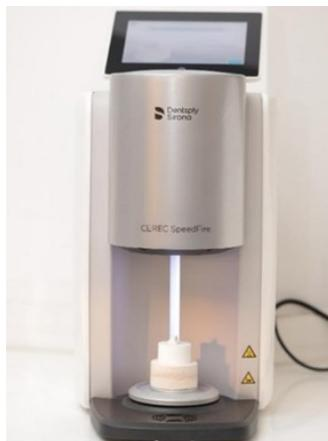
**Figure (3):** CEREC speed fire furnace for speed sintering of zirconia
