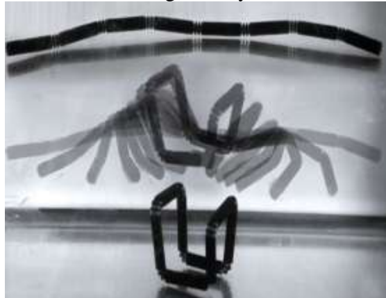
Figure 1: Transformation of 1D structure to 3D structure in Water
