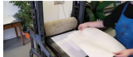
(Figure 29) Placing the paper and the plate in the printing machine
