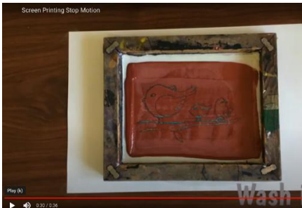
(Figure 17) A shot showing covering the silkscreen with the resistant substance
