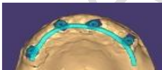
Figure 3: CAD design of the bar substructure.
