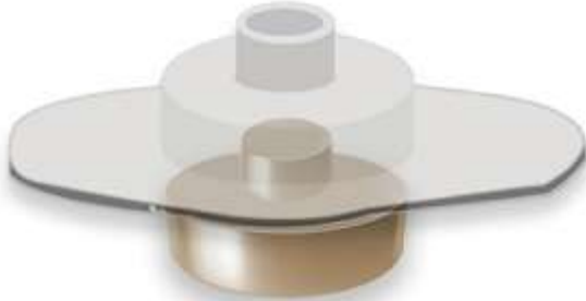
Figure (1): Plastic mold used for condensation of veneering porcelain powder over the ceramic disks. 1. Plastic mold. 2. Veneering porcelain. 3. Plastic wing to increase mold stabilization and easier handling. 4. Ceramic disk.
