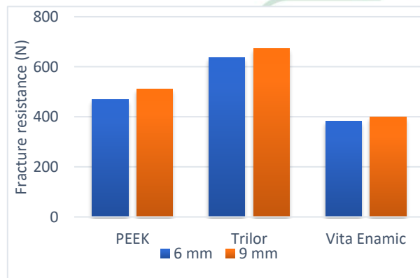
Figure 2: Bar chart showing average fracture resistance (N) for different post materials and lengths (B)
