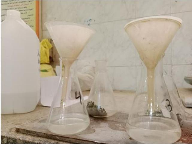
FIGURE 7. The filtration process for the concrete solution
