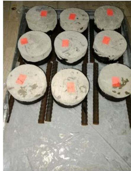
FIGURE 6. Sorptivity Test
