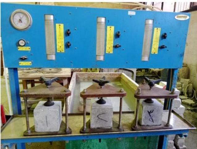
FIGURE 5. The water pressure applied to the samples
