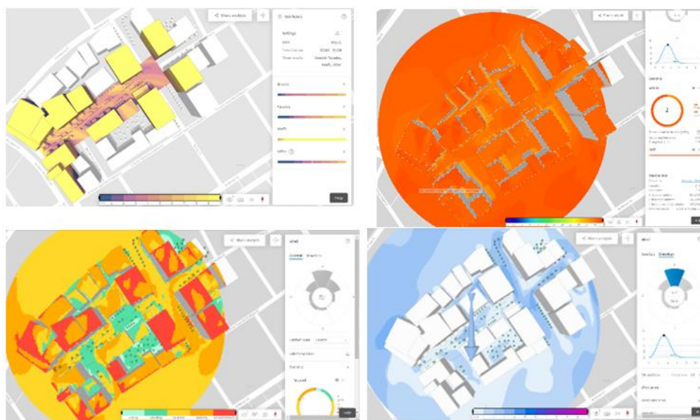
FIGURE 9. [A,B,C,D] A The layout [upper left] shows the Solar analysis, B [upper right] shows the thermal comfort index during July 15, C [lower left] shows the wind comfort analysis for performing activities, D [Lower right] shows the wind analysis, after adding vegetation and applying shades along
