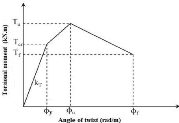
Fig. 21 Calculation of the ductility ratio.
