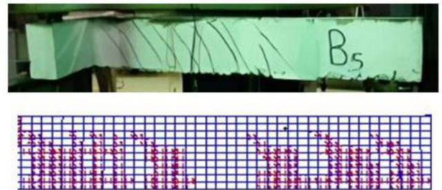
**Fig 13** Comparison between The FEA Failure modes and crack patterns of the verification model with experimental results.
