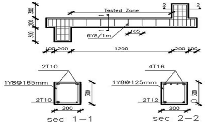
**Fig 8.** Geometry, beam reinforcement and section details.
