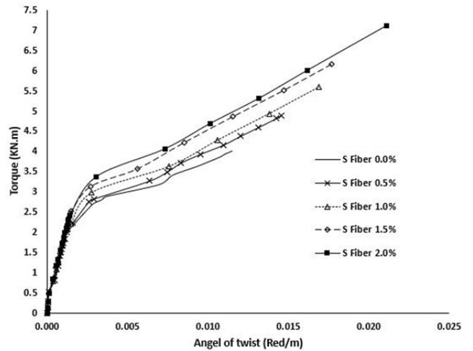
Fig. 18 Effect of steel fiber ratio on Torque- Angel of twist relation.
