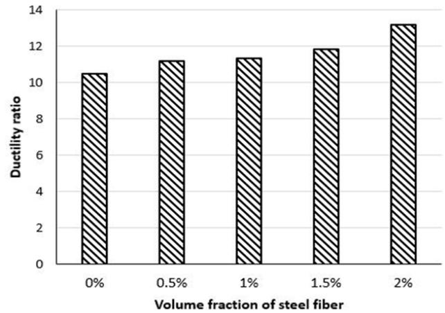
Fig. 22 Effect of steel fiber on the ductility ratio of specimens.
