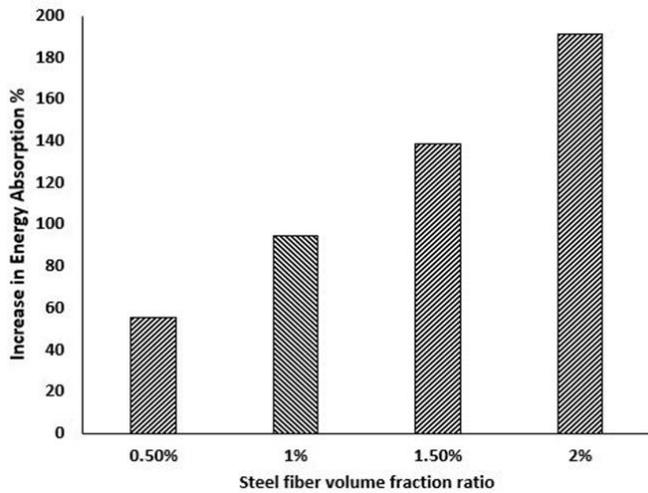
Fig. 20 Influence of adding steel fibers to SCC beams on energy absorption.
