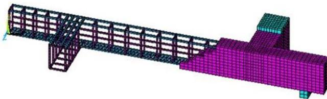
**Fig. 5** ANSYS model of concrete and reinforcement meshing of present verification model.
