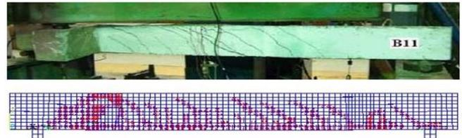
**Fig 7** Comparison between The FEA Failure modes and crack patterns of the verification model with experimental results by Khaled S. [16].
