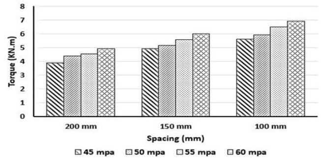
Fig 15 Effect of spacing between stirrups.
