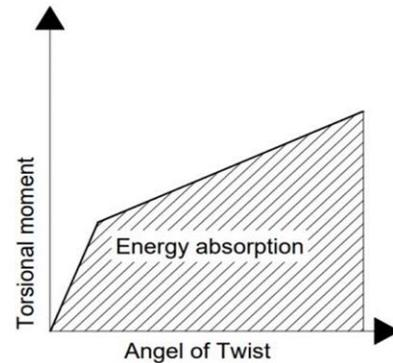
Fig. 19 Energy absorption in the torsional moment – the angle of twist curve.
