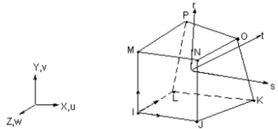
**Fig. (1)** Solid 65 element 3-D Reinforced Concrete in ANSYS [19].
