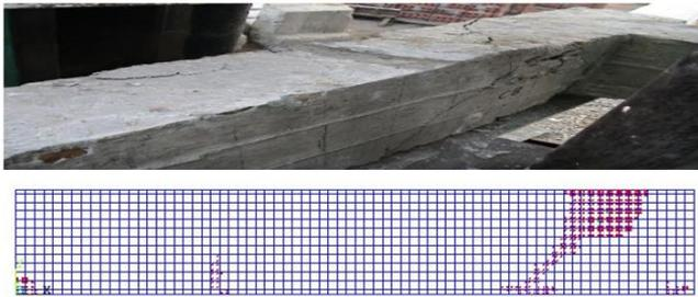
**Fig 11** Comparison between The FEA Failure modes and crack patterns of the verification model with experimental results.
