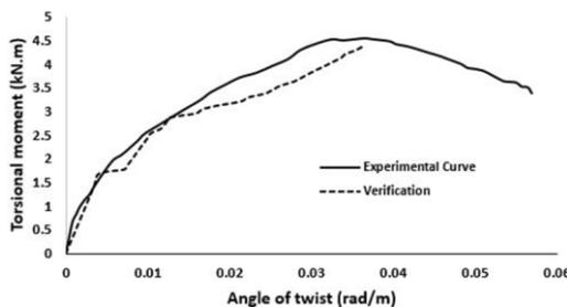
**Fig 6** Comparison between the current study verification model and the experimental by Khaled S.[16].
