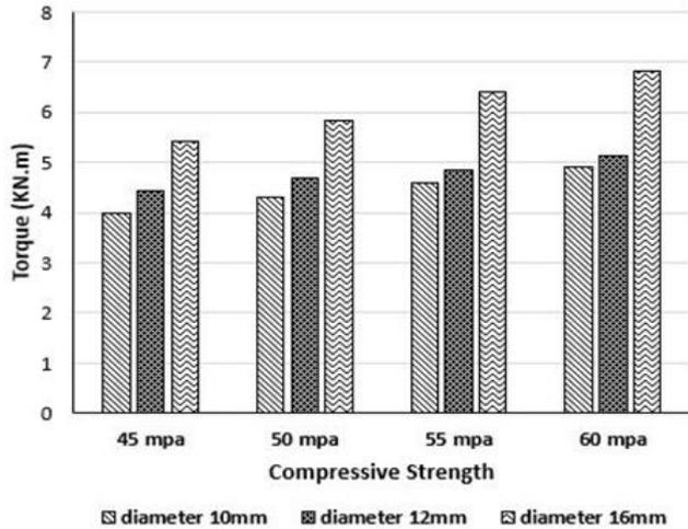
Fig 17 The effect of longitudinal reinforcement ratio on the torque of the SCC beam.
