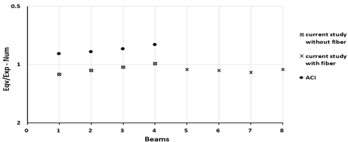
Fig 23 The application of the proposed equation with the results of the present analytical study for SCC beams with and without steel fiber addition
