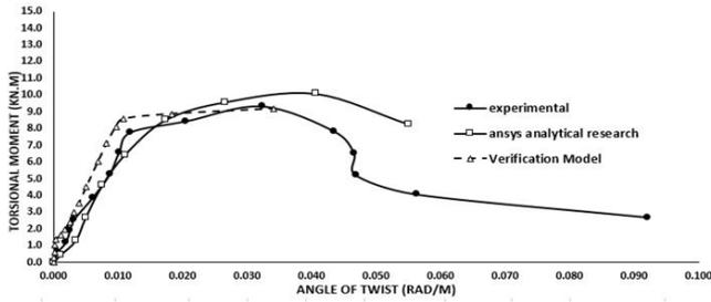
**Fig 10** Comparison between the torque-angle of twist relationship reported in the experimental study [21] and the verification model
