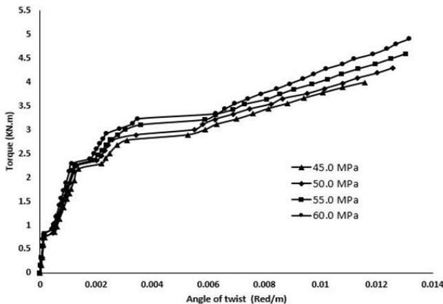
Fig 14 Effect of compressive strength on Torque- Angel of twist relation
