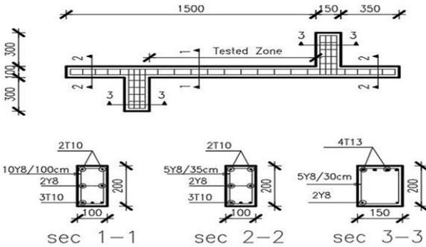
**Fig. 4** Geometry, beam reinforcement and sections details of verification model, Khaled [16].
