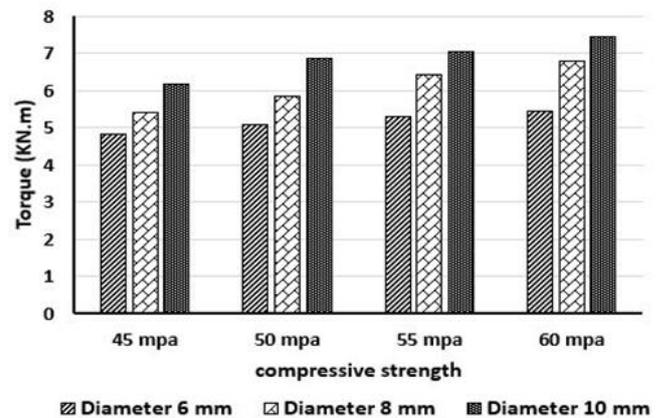
Fig. 16 The effect of stirrups diameter on the torque of the SSC beam.
