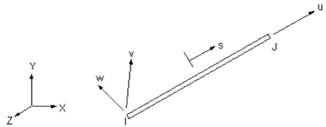
**Fig. (2)** Element Link 180 (Steel Reinforcement) in ANSYS [19].
