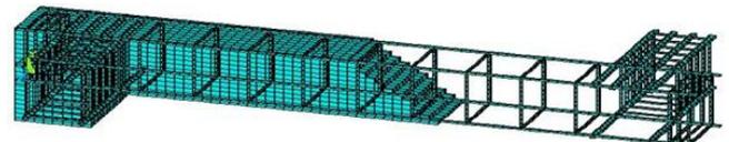
**Fig 9.** Present verification model simulation with steel reinforcement and meshing.
