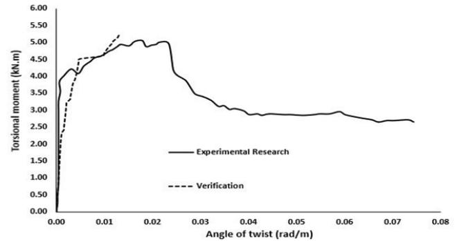
**Fig 12** The torsional-twisting comparison between the experimental [16] and current verification model.
