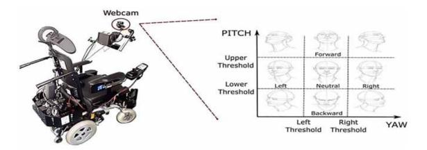
Fig.11. Electric wheelchair with an installed webcam for face detection and orientation estimation [5].
