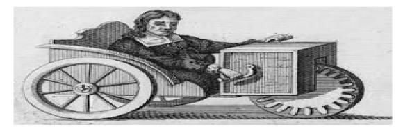
Fig. 2: Depicts Stephan Farfler's invention in 1655, the first self-propelled wheelchair with three wheels, allowing users to move it independently using a rotary handle.
