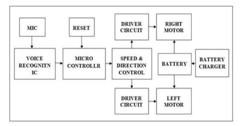
Fig. 10: Block Diagram of voice-controlled wheelchair for physically challenged people
