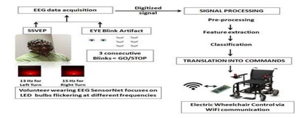
Fig. 13. Schematic diagram of the proposed SSVEP and eye blink based electric wheelchair control technology [60]
