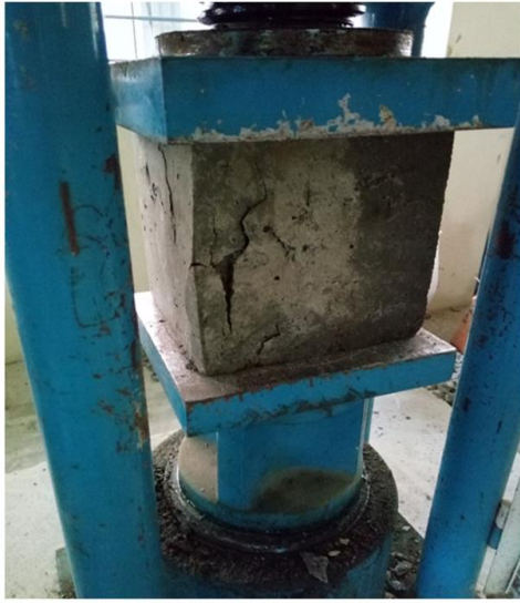
Figure 5: Broken Specimen after Reach Ultimate Load
