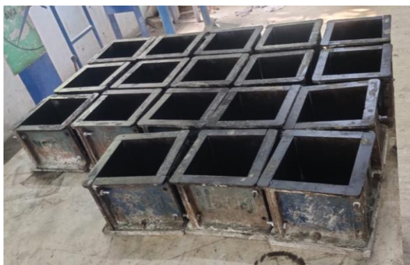
Figure 3: Preparing of Cube Moulds
