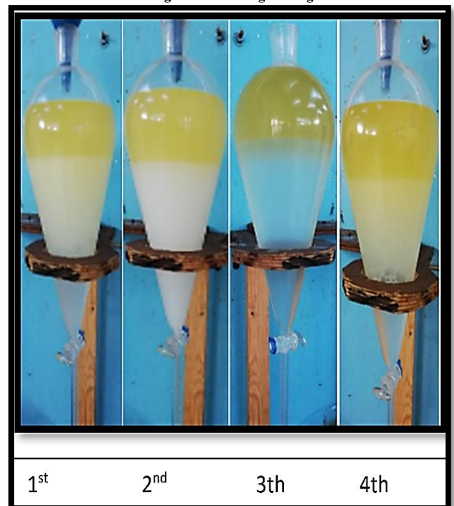
Figure 7. Stage of washing biodiesel.
