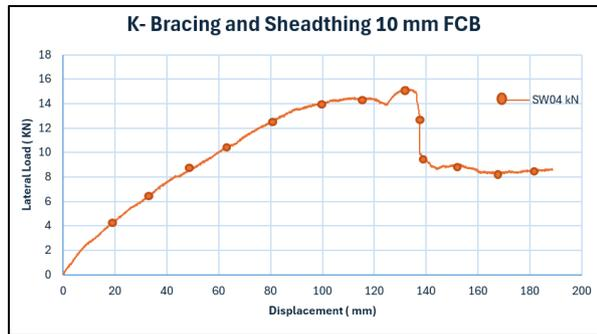
Figure (27): Effect of K-bracing and sheath specimen.
