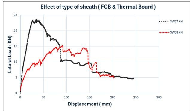
**Figure (31):** Effect of type of sheath specimen.
