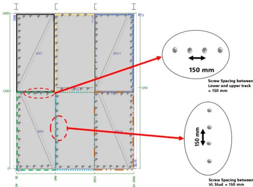
Figure (12): Shear Wall (1800\*2400 mm) Sheath with Thermal Board 20 mm.
