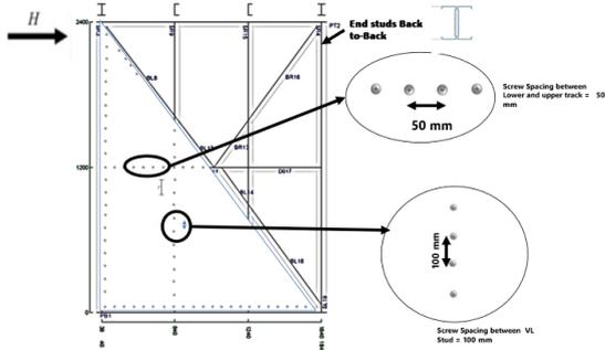
Figure (11): Shear Wall (1800\*2400 mm) Sheath with Fiber Cement Board 10 mm.
