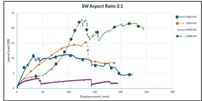
Figure (33): Effect of Shear walls with Aspect Ratio 2:1.
