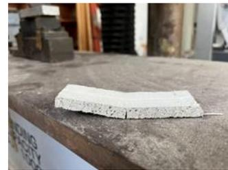
Figure (6): Bending test for thermal board and fiber cement board.
