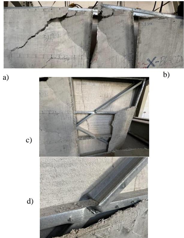
a) split screw board      b) crushing board
