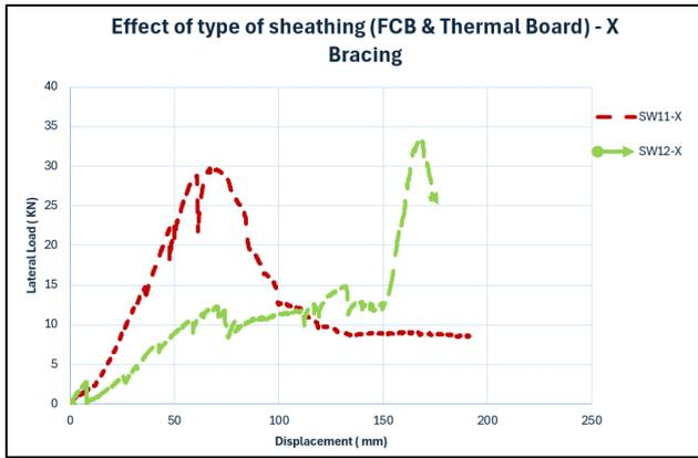
Figure (33): Effect of type of sheath and X-Bracing specimen.
