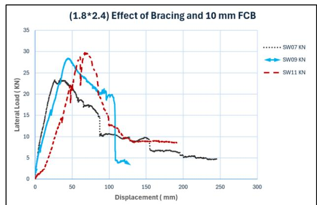
Figure (29) : Effect of bracing and FCB specimen.
