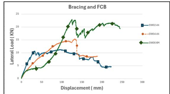
Figure (25): Effect of bracing and FCB (SW02, SW04, SW06) specimens.
