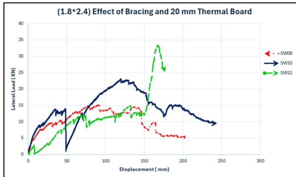
**Figure (30) :** Effect of bracing and thermal board specimen.
