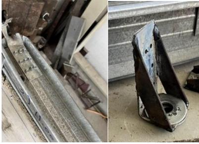
Figure (15) ; The old HD and Modified one with stiffener.
