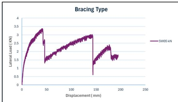
Figure (24): Effect of bracing on SW05 specimen.
