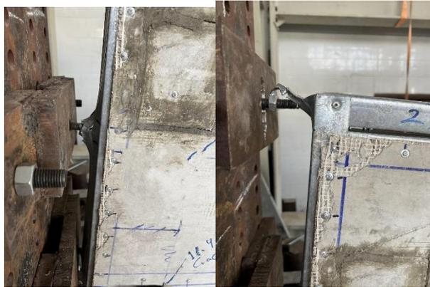
(a) Pull out HD before modified. (b) Uplift and pull-out tension stud.
