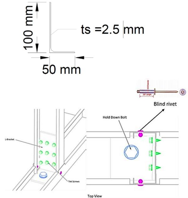
Figure (3): Hold Down Fixation with back-to-back Stud.
