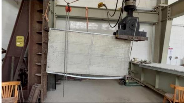
Figure (16): The Shear wall SW04-K after the test under monotonic test before strength the lower track with Modified HD-1.
