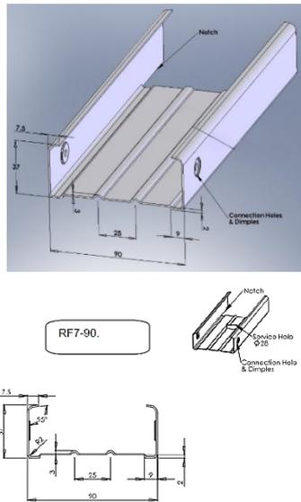
Figure (1): Dimension for Section (RF7-090).
