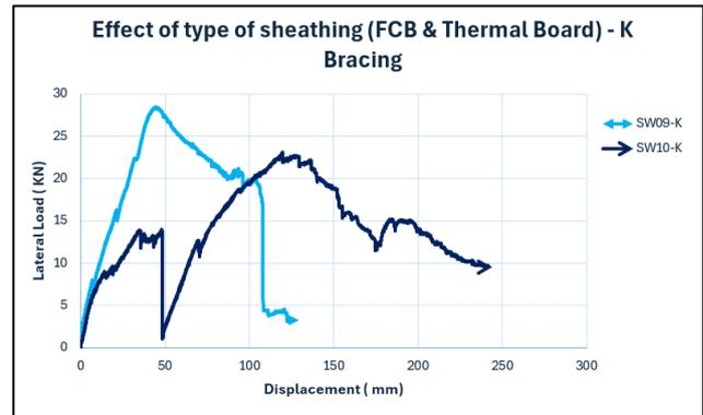
**Figure (32):** Effect of type of sheath and K- Bracing specimen.
