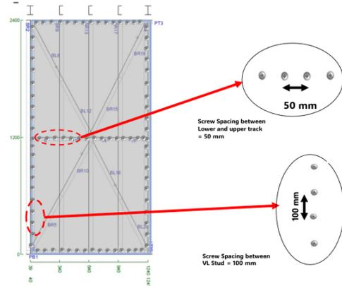
Figure (13): Shear Wall (1200\*2400 mm) Sheath with Fiber Cement Board 10 mm.
