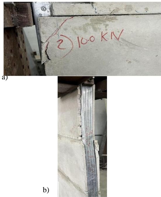
a) board cracks      b) top track buckling
