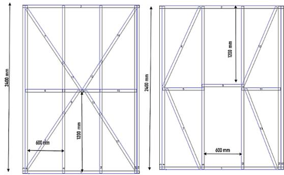
Figure (5): Shear walls Frame 1200\* 2400 mm and 1800\*2400 mm.
