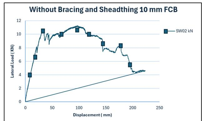
Figure (26): Effect of sheath for SW02 specimen.
