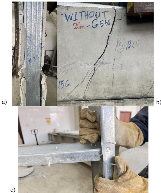
a) buckling upper track, b) Thermal board cracks
