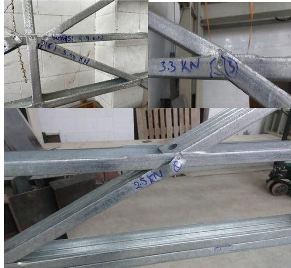
Figure (18): Failure modes of Specimen SW05-X.
