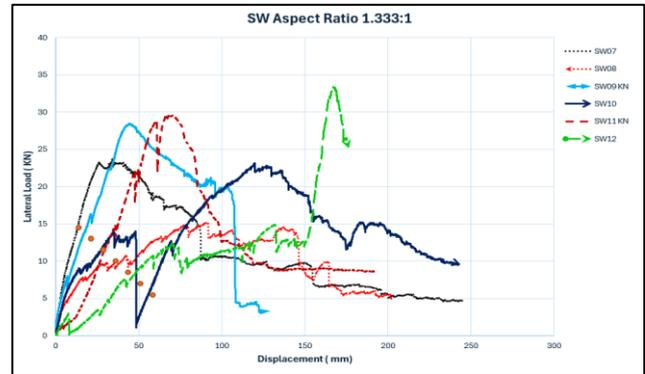
Figure (34): Effect of Shear walls with Aspect Ratio 1.333:1.
