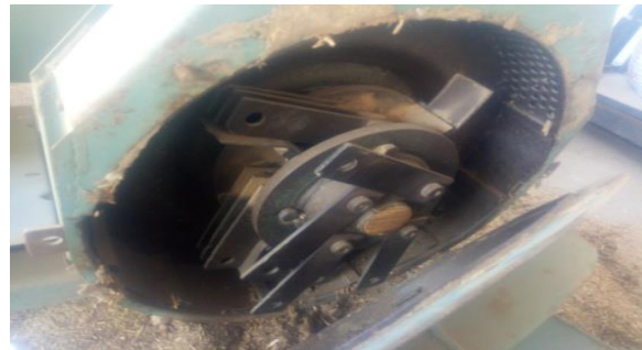
Fig. (2): The cutting head of the hammer mill machine
