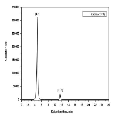
Fig.2A. The HPLC radiochromatogram of  $[^{99m}Tc]$ tricarbonyl precursor, atRt = 4.7 min and free  $[^{99m}Tc]$ pertechnetate at Rt = 11.5 min.
