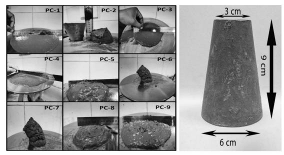
Fig. 6 Photographic pictures for initial flow test of PCE-based SPs grout samples
