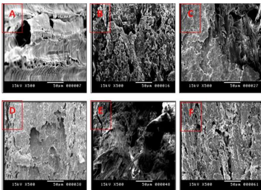
Fig 4. SEM micrographs for the cross-section magnified ( $\times 500$ ) of samples treated after aging compared to the standard samples, (A) Standard (B) Klucel E 1% (C) Klucel 1% / Nano cellulose 3% (D) Klucel 1% / Nano cellulose 5% (E) Klucel 1%/Nano clay 3% (3) Klucel 1%/Nano clay 5%
