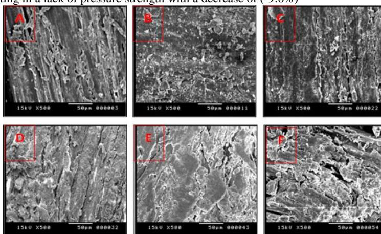
Fig 3. SEM micrographs for the tangential section magnified ( $\times 500$ ) of samples treated after aging compared to the standard samples, (A) Standard (B) Klucel E 1% (C) Klucel 1% / Nano cellulose 3% (D) Klucel 1% / Nano cellulose 5% (E) Klucel 1%/Nano clay 3% (F) Klucel 1%/Nano clay 5%
