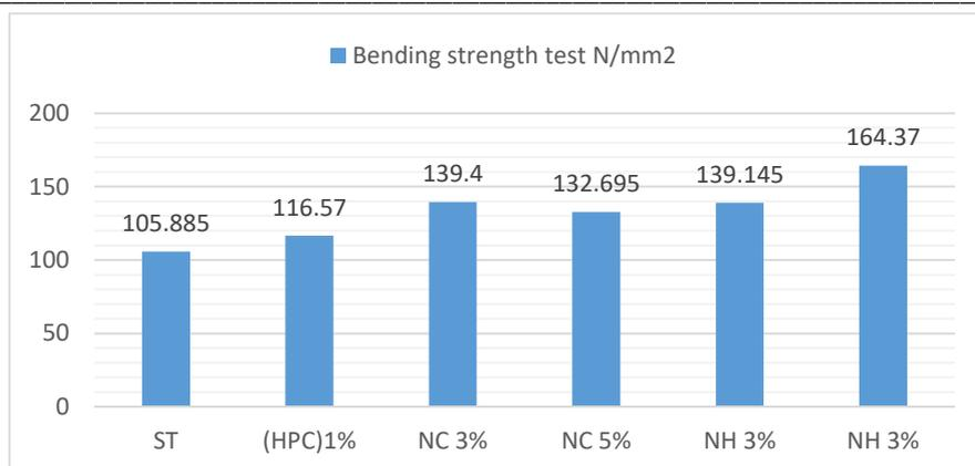
Fig 6. Bending strength test results show increasing bending strength in the presence of a mixture of Klucel 1%/Nano clay 5% presence of Nano cellulose (NC).
