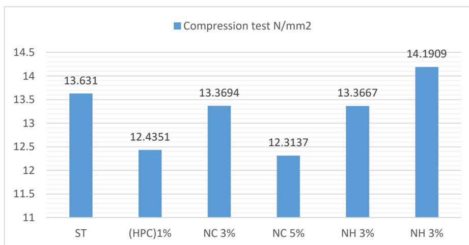
Fig 5. Compression test results show increasing compression strength in the presence of a mixture of Klucel 1%/ Nano clay 5%
