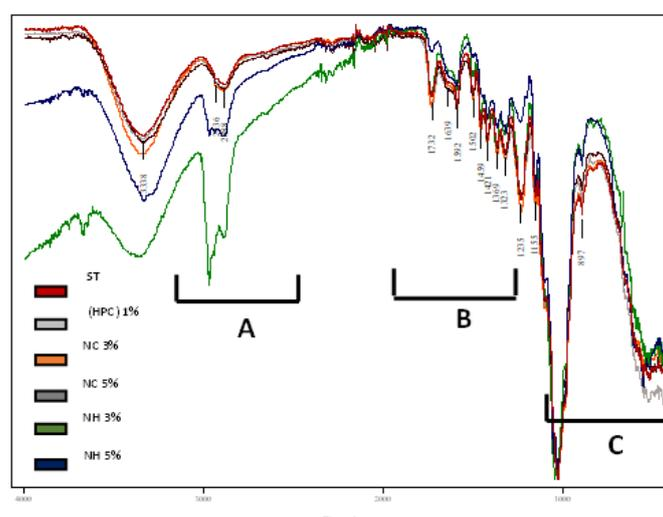
**Fig 1.** Infrared spectroscopy of the treated samples after aging (thermal - Photo) compared to the standard samples and Signed with three regions (A-B-C) of wavelength from (400-4000 cm<sup>-1</sup>)
