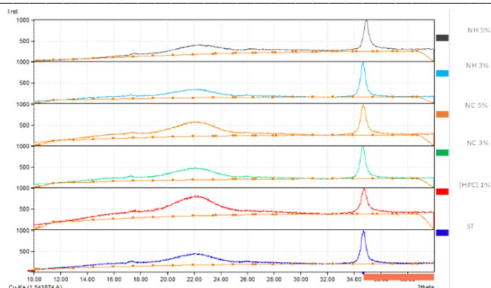
Fig 2. X-ray diffraction pattern of samples treated after aging (thermal-photo) compared to the standard sample to determine the degree of crystallinity in cellulose.
