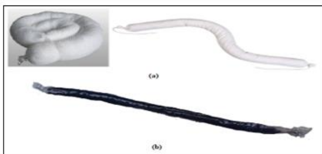
FIGURE 13. Developed Model (a) before and (b) after immersing in Oil/Water Mixture
