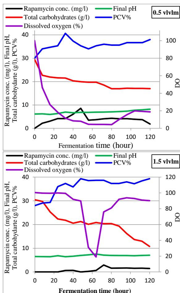
**Fig. 7:** The profile of fermentation conducted in 7.5-litre fermentor for rapamycin production at 600 rpm and aeration rates of 0.5 and 1.5 v/v/m.
