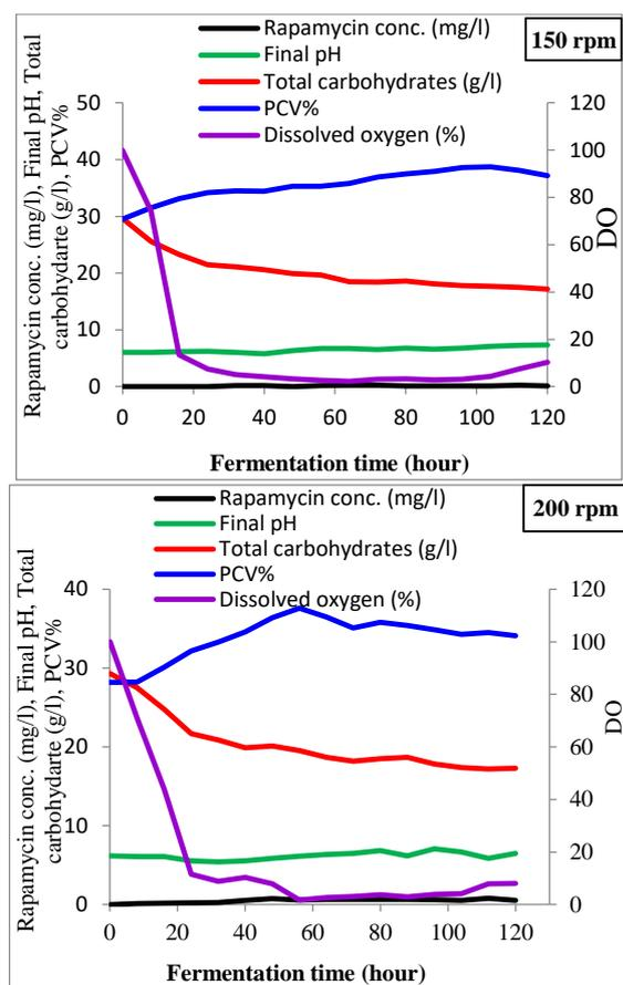
**Fig. 2:** The profile of fermentation conducted in 7.5-litre fermentor for rapamycin production at agitation speed of 100, 150 and 200 rpm.
