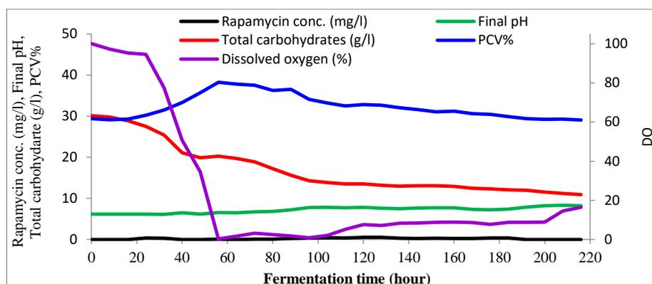
**Fig. 3:** The profile of fermentation conducted in 7.5-litre fermentor for rapamycin production at agitation speed of 400 rpm.
