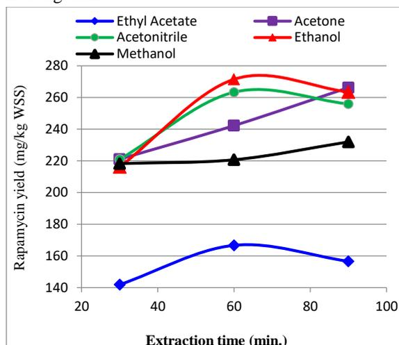
**Fig. 8:** Extraction of rapamycin from wet solid suspends (WSS) by different organic solvents applied for different times.
