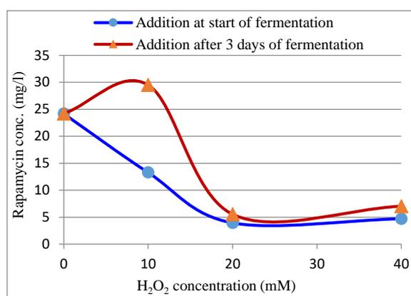
**Fig. 5:** Production of rapamycin at different supplements of H<sub>2</sub>O<sub>2</sub> added at start or after 3 days of fermentation start.
