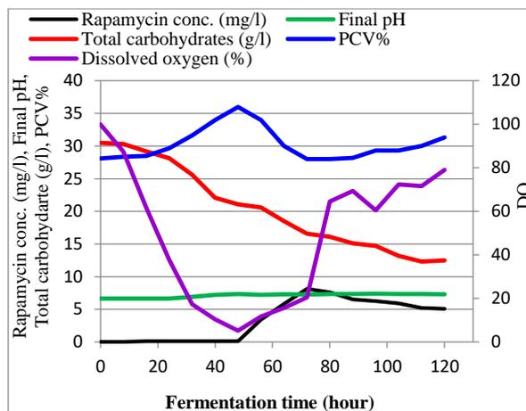
**Fig. 6:** The profile of fermentation conducted in 7.5-litre fermentor for rapamycin production at agitation speed of 600 rpm.
