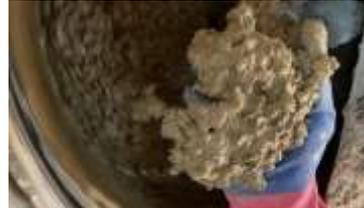
Fig. 4: Fresh geopolymer concrete
