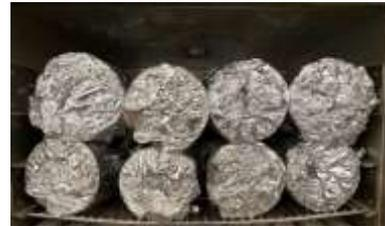
Fig. 5: Oven heat-curing of geopolymer concrete specimens
