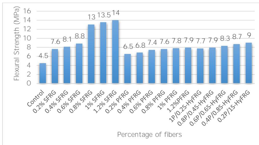
Fig.9: Flexural strength values of the investigated mixes.
