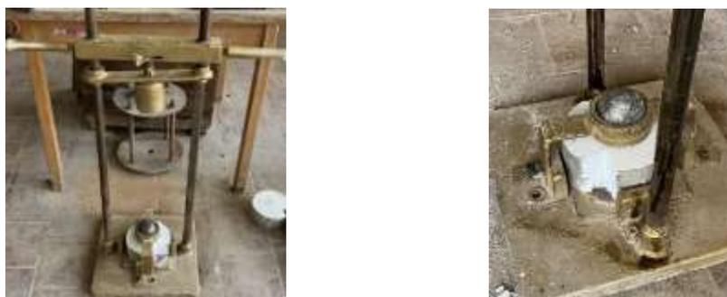
Fig.6: Falling weight collision test
