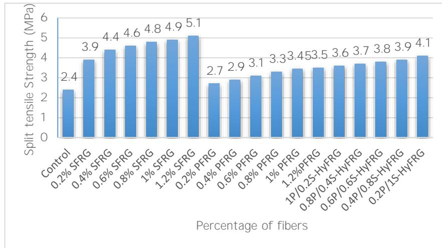
Fig.8 Indirect tensile strength values of the investigated mixes.
