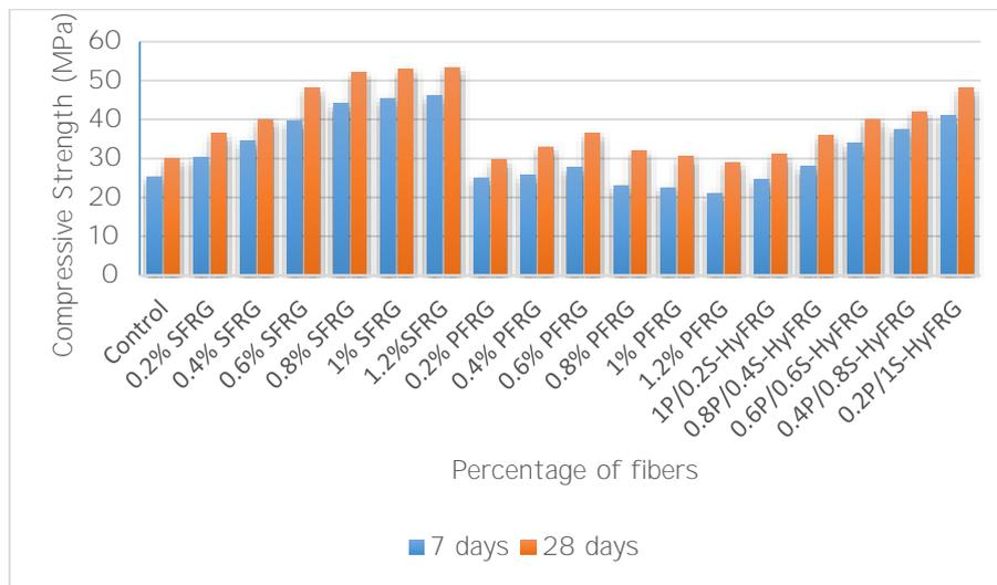
Fig. 7: Compressive strength values of the investigated mixes.
