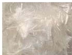
**Fig. 2: Polypropylene Fibers**
