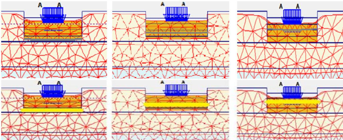
**Fig. 5: Strip footing soil model deformed shapes under uniform distributed load at different geogrid depth, ( $D_g/H$ )**
