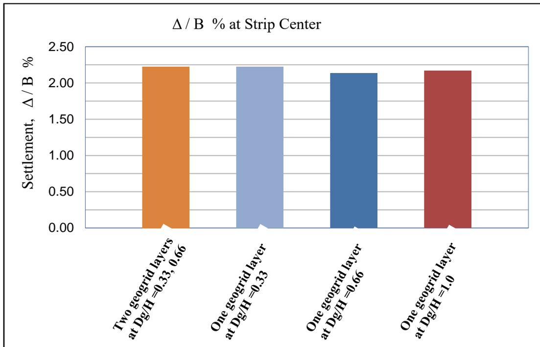
Fig. 7: Normalized vertical settlement below centerline of loaded strip footing at varies geogrid depth, (Dg/H)
