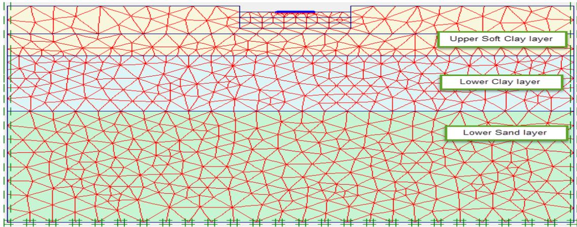
Fig. 3: Finite element mesh geometry and boundaries for strip footing soil model
