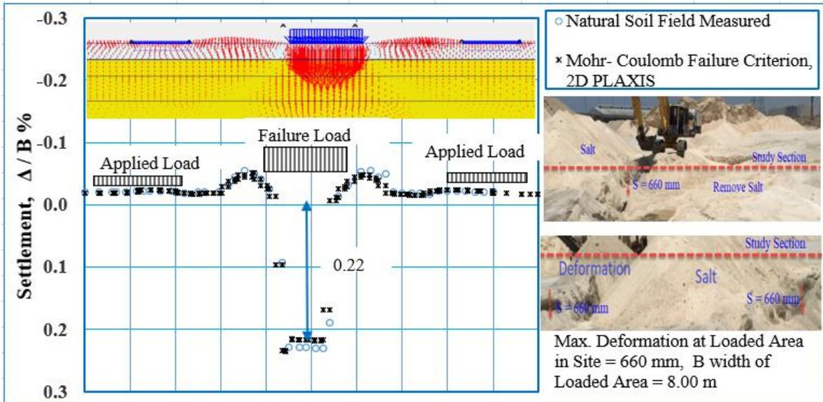
Fig. 2 : Normalized vertical displacement at failure load step, to ensure section1 Field measured and recorded.
