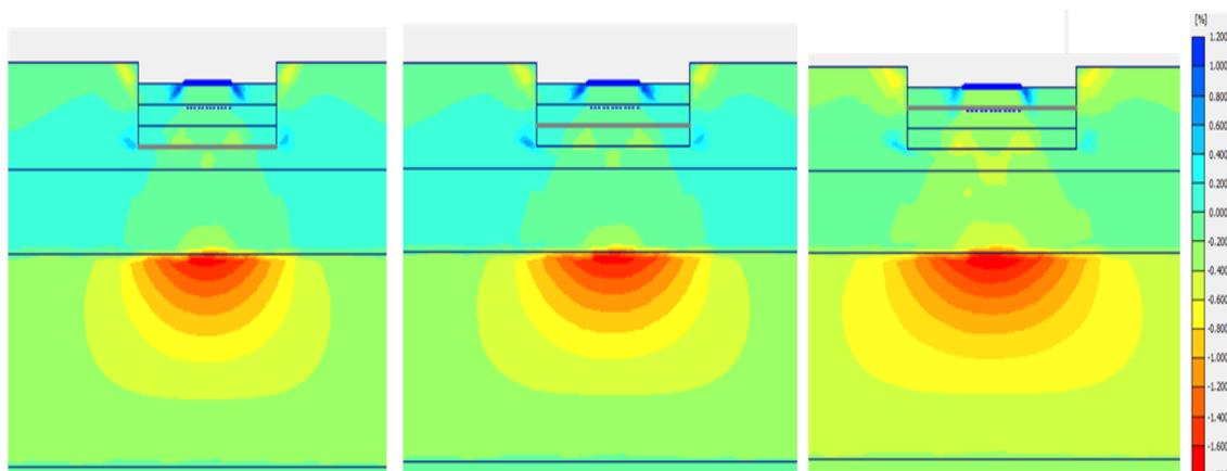
**Fig. 6: Strip footing soil model strain at different geogrid depth, ( $D_g/H$ )**
