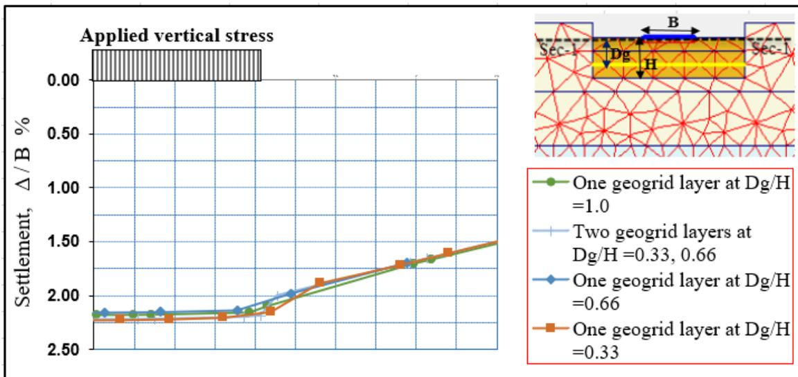
Fig. 4: Variation normalized vertical settlement below the loaded strip footing at different geogrid depth, ( $D_g/H$ )
