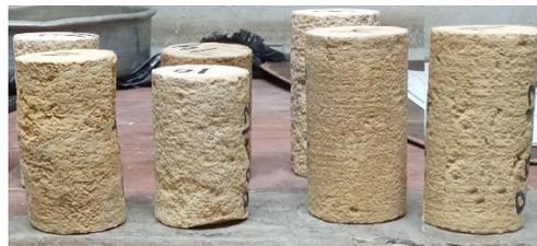
Fig. 3 Shape of the Cylinders Samples of Sandstone rocks
