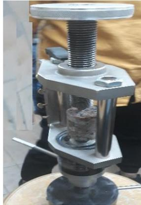
Fig. 6 Photograph showing the Point load test system
