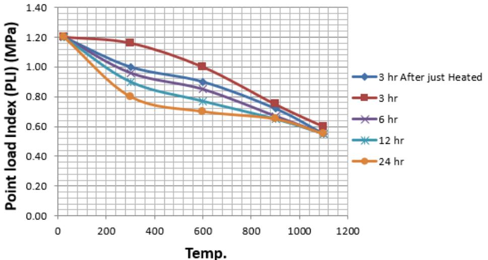
Fig. 9. Variation of the (PLI) (MPa) of Marble rock for different temperature degrees in different cases
