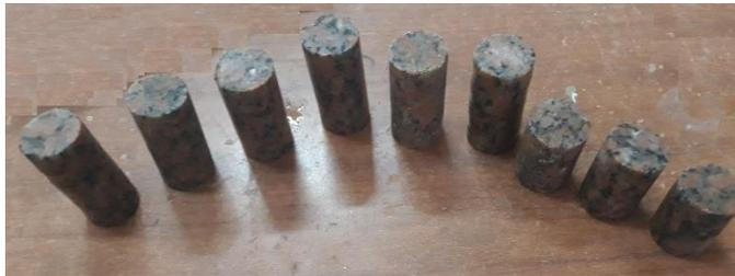
Fig. 2 Shape of the Cylinders Samples of Aswan Granite rocks
