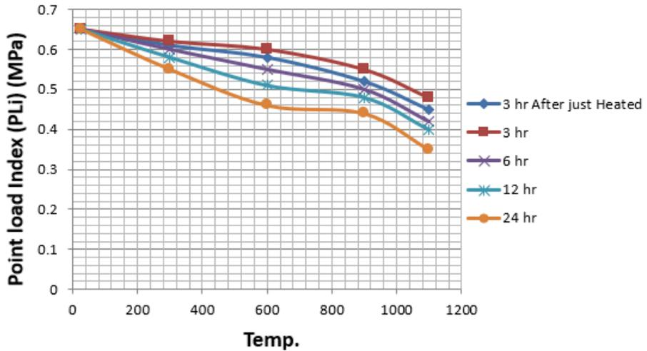
Fig. 8. Variation of the (PLI) (MPa) of Limestone rock for different temperature degrees in different cases
