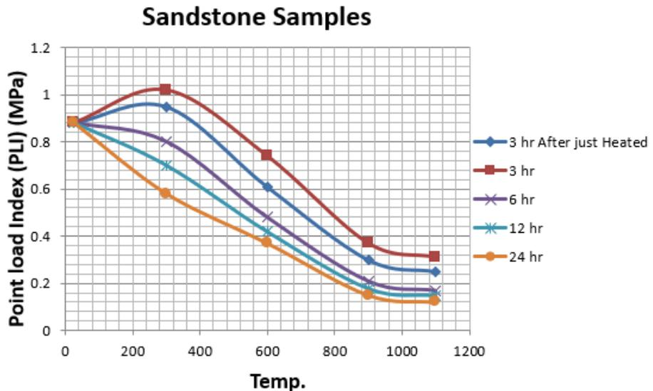
Fig. 7. Variation of the (PLI) (MPa) of Sandstone rock for different temperature degrees in different cases
