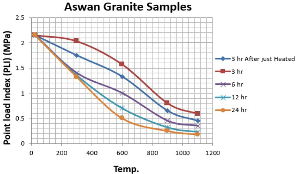
Fig. 6. Variation of the (PLI) (MPa) of Aswan granite rock for different temperature degrees in different cases
