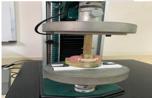
**Figure (7):** Testing for retention with universal testing machine.
