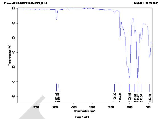
**Figure 3:** FTIR sample for the untreated silicon elastomer specimens.
