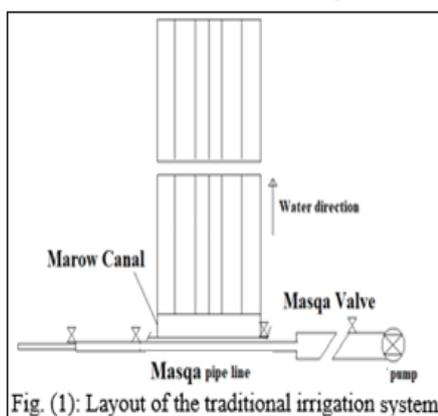
Fig. (1): Layout of the traditional irrigation system
