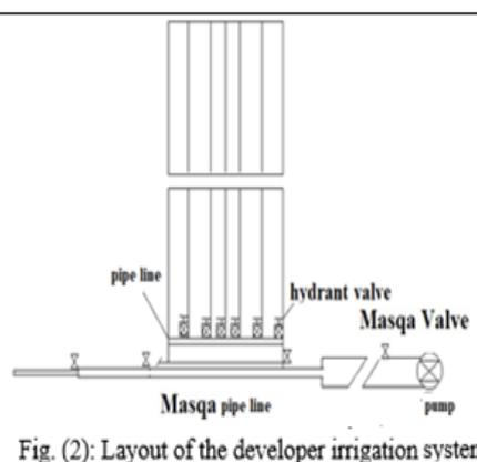
Fig. (2): Layout of the developer irrigation system
