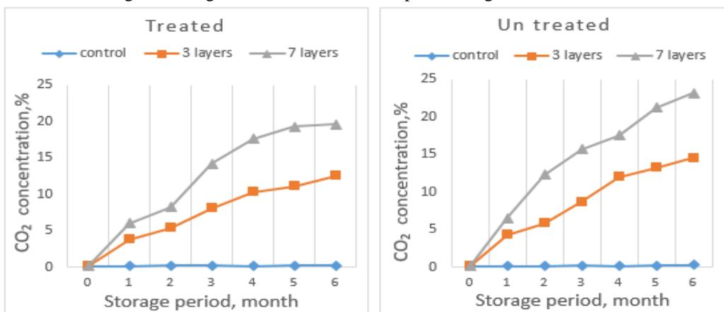
**Fig. 8. Carbon dioxide concentration as function to storage period for various types of bags.**
