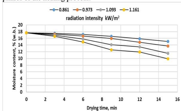
**Fig. 3. the variation in moisture content of corn grain to the duration of drying time under varying radiation intensity levels.**
