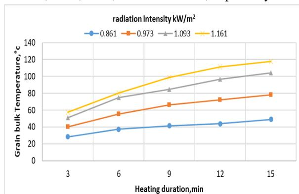
**Fig. 4. Effect of different radiation intensity grain bulk temperature.**
