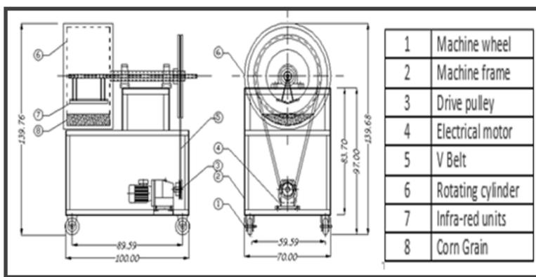
Fig. 1. Schematic diagram for the rotary Infra-red heating unit
