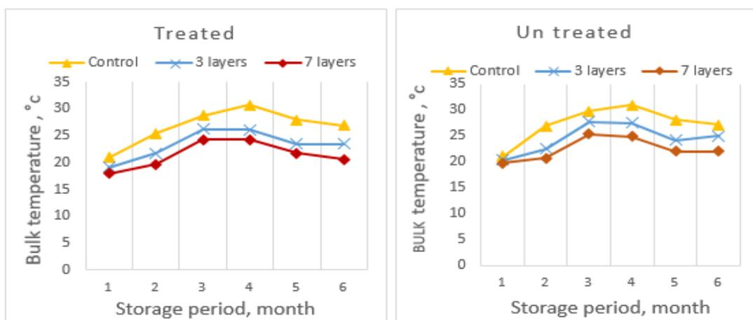
**Fig. 6. Grain bulk temperature as related to storage time for the heat-treated grain stored in different types of bags.**
