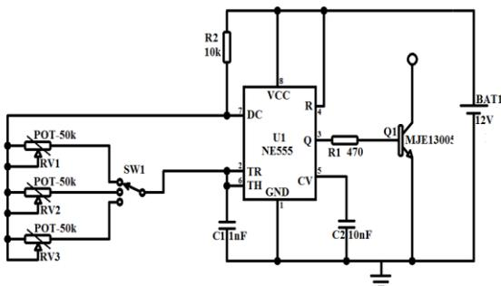
Fig. 1. Ultrasonic generator circuit
