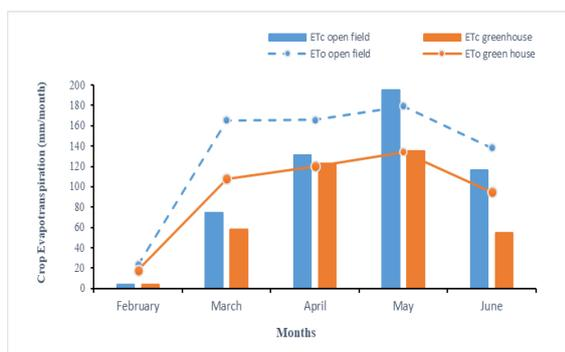
**Figure 4. Relationship between  $ET_o$  and  $ET_c$  inside greenhouse and outside cultivation.**
