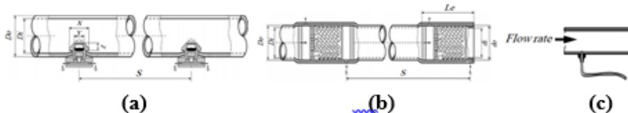
**Figure 2.** A schematic types of the used devices for (a) on-line, (b) built-in and (c) micro-tube emitter.
