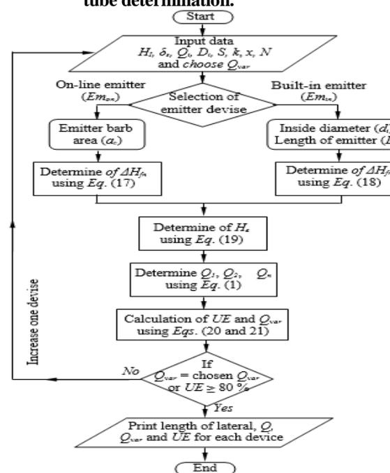
**Figure 4.** Software model flow-chart for the best length of micro-irrigation laterals using different devices determination.
