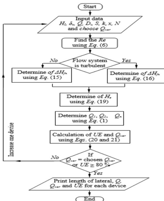
**Figure 3.** Software model flow-chart for the best length of micro-irrigation laterals using micro-tube determination.
