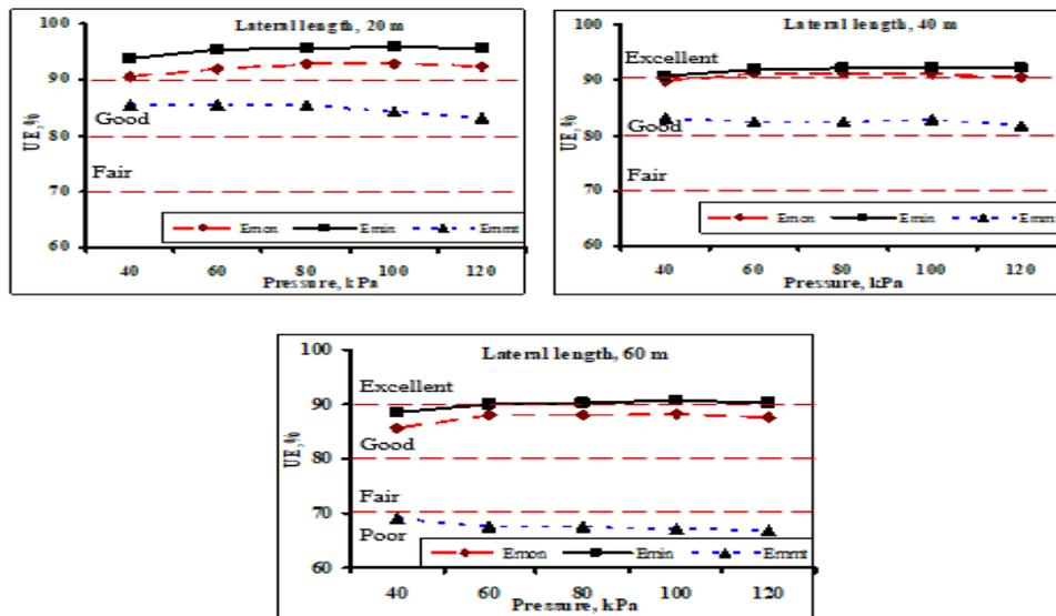
**Figure 6. Influence of pressure and lateral lengths on uniformity emission of different devices.**
