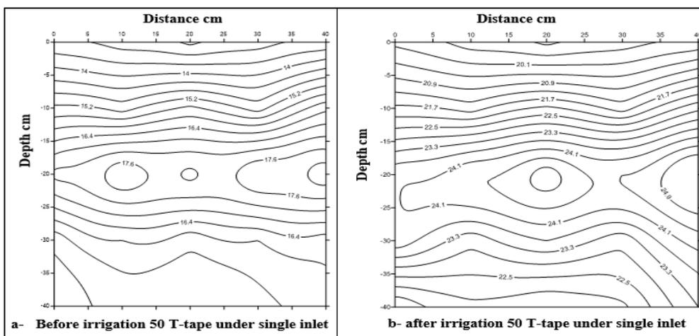
**Fig. 8. Soil moisture distribution (a) before and (b) after irrigation under using single inlet with T-tape lateral under lateral length 50 cm.**
