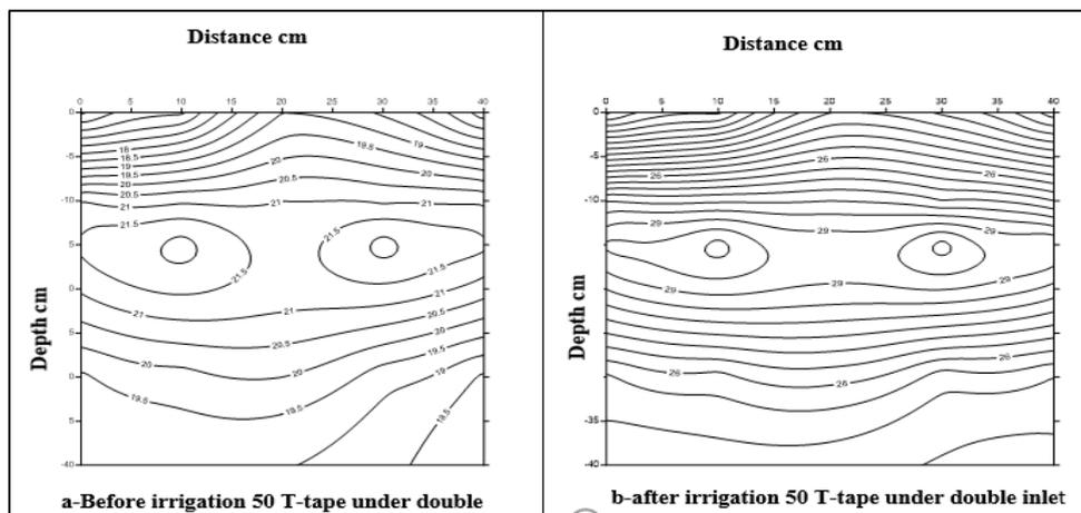
**Fig. 6. Soil moisture distribution (a) before and (b) after irrigation under using double inlet with T-tape lateral under length of lateral 50 cm.**
