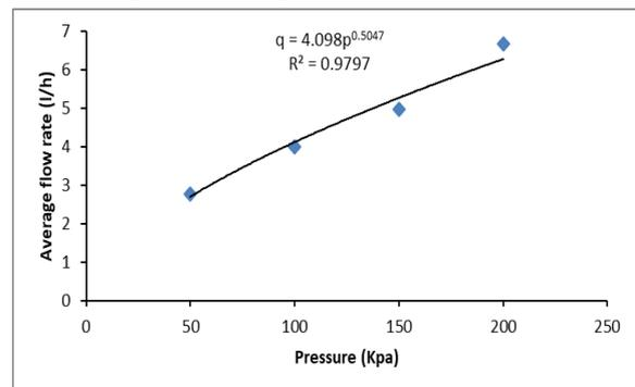
**Fig. 3. Linear regression for 4 L/h pressure GR emitter characteristic curve**
