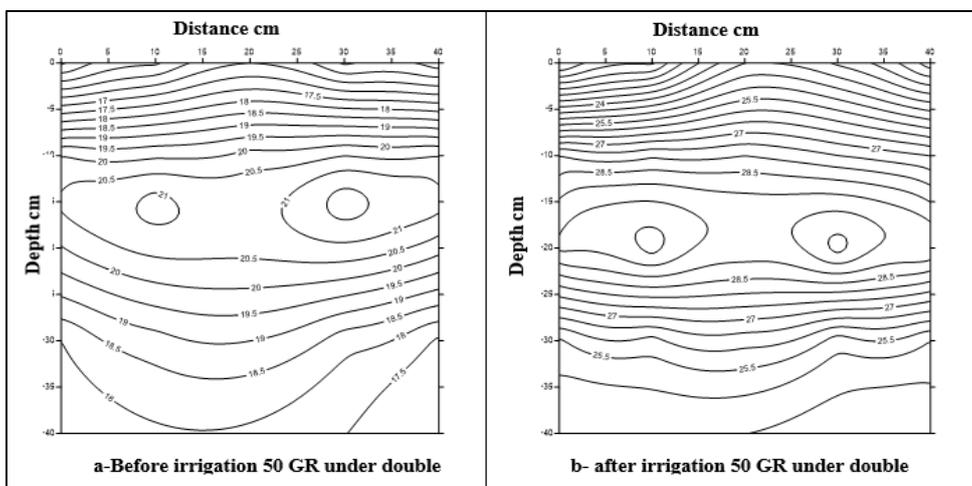
**Fig. 7. Soil moisture distribution (a) before and (b) after irrigation under using double inlet with GR lateral under length of lateral 50 cm.**
