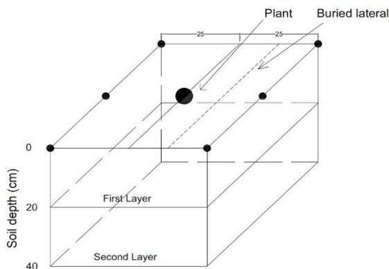
**Fig. 2. Location of soil samples with 8 spots at each soil layer in determining soil moisture distribution with depth for each treatment**
