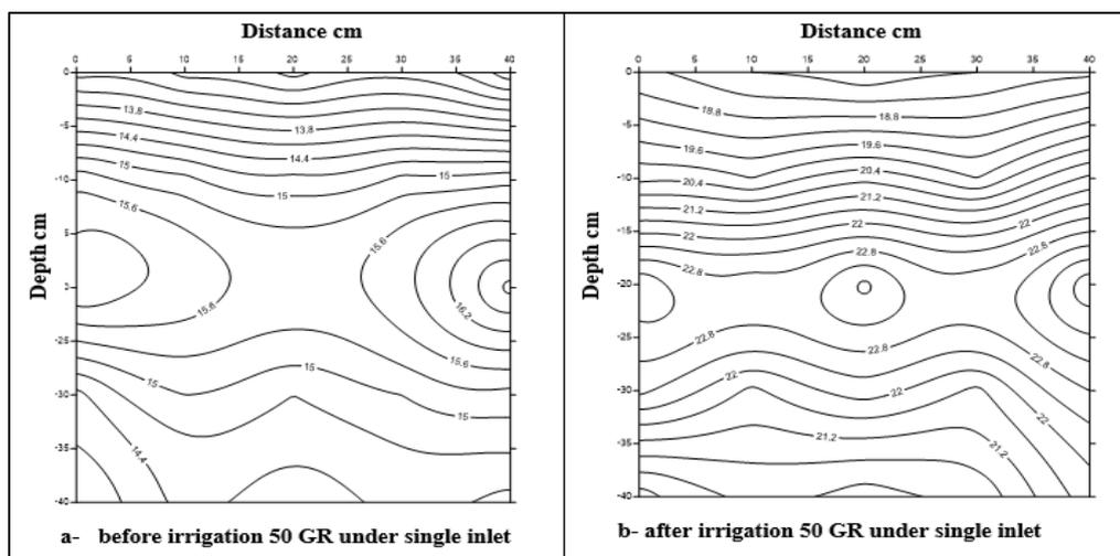
Fig. 9. Soil moisture distribution (a) before and (b) after irrigation under using single inlet with GR lateral under lateral length 50cm.
