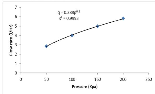
**Fig. 4. Linear regression for 4 L/h pressure GR emitter characteristic curve.**
