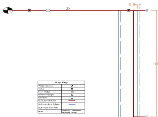
**Fig. 1. Experimental layout of the sub surface drip irrigation system (Single inlet- Double inlet)**
