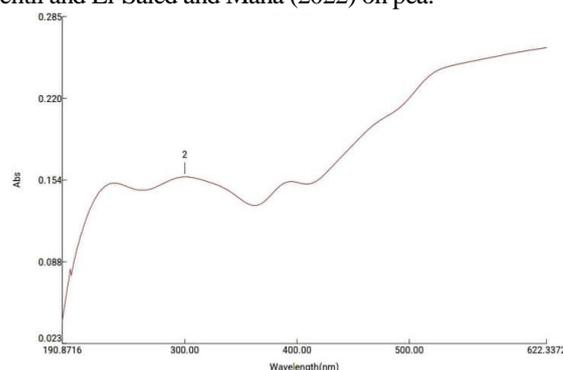
**Figure 4. ZnO nanoparticles analysis via spectrophotometer. The UV-vis absorbance spectrum of zinc oxide nanoparticles from 190 nm to 1100 nm.**
