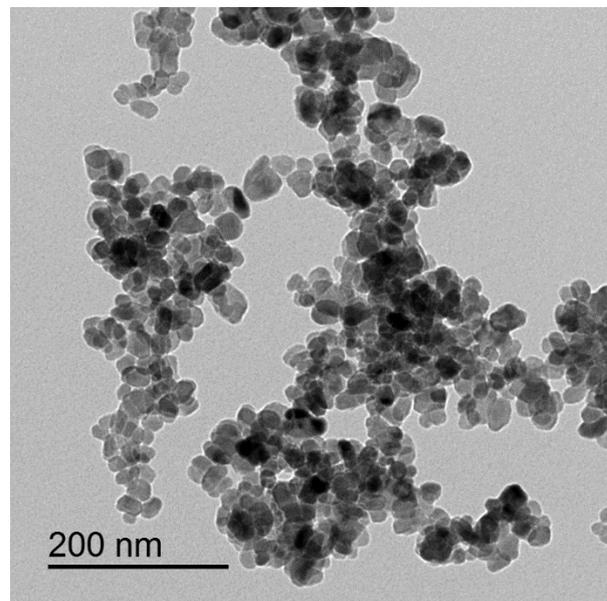
**Figure 1. Physical characterization of ZnO nanoparticles using TEM.**
