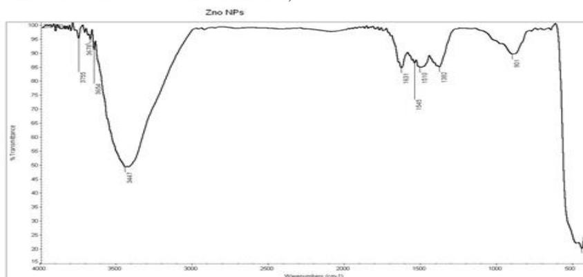
**Figure 3. Analysis of ZnONPs utilising infrared spectroscopy with the Fourier transform. The surface functional group and structure of the ZnO NPs were revealed by the FTIR spectra.**
