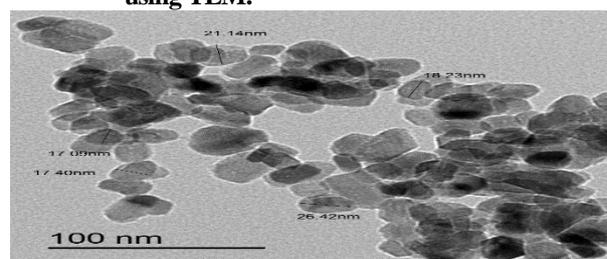
**Figure 2. TEM revealed both ZnO NPs small round nanoparticles and big rod nanoparticles.**
