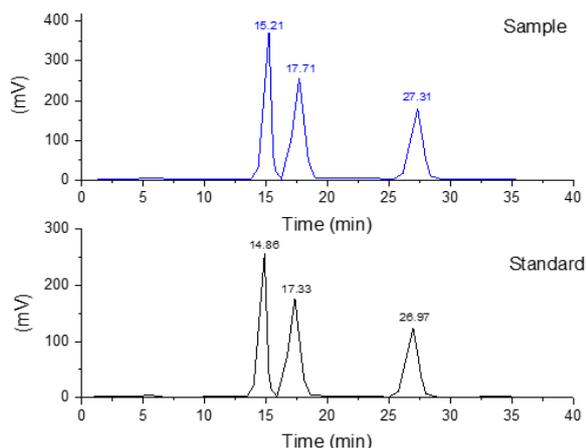
**Figure 1. HPLC profile of fructose, glucose, and sucrose standard compounds and pomegranate granules ingredients sample**
