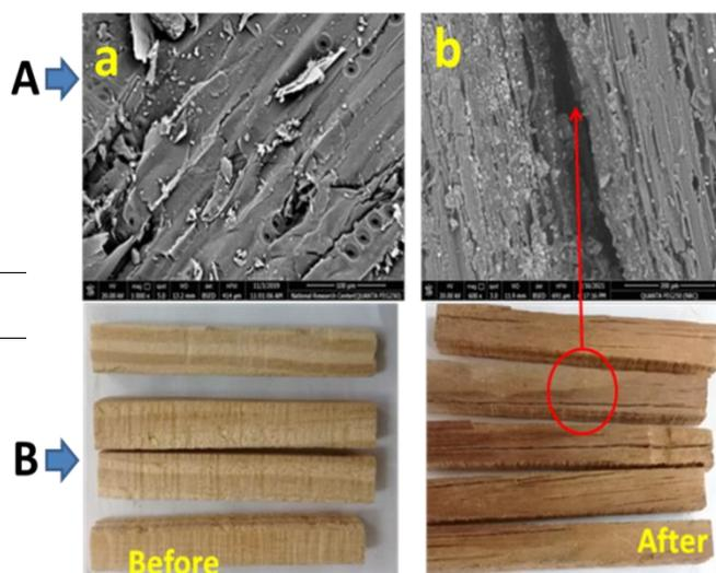
Fig. 2: A) SEM of the experimental wood a) before, b) after heat treatment.
