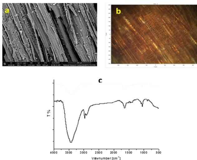
**Fig. 1:** a) Scanning electron microscopy, b) lighting microscope, and c) FTIR of Heritage wood.
