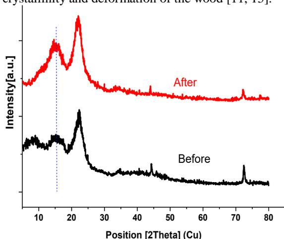
Fig. 4: X-ray diffraction of the experimental wood before and after heat treatment.
