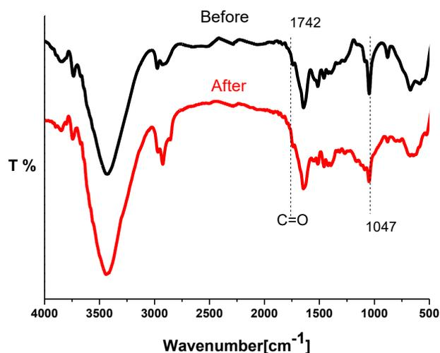
Fig. 3: FTIR of the experimental wood before and after heat treatment.
