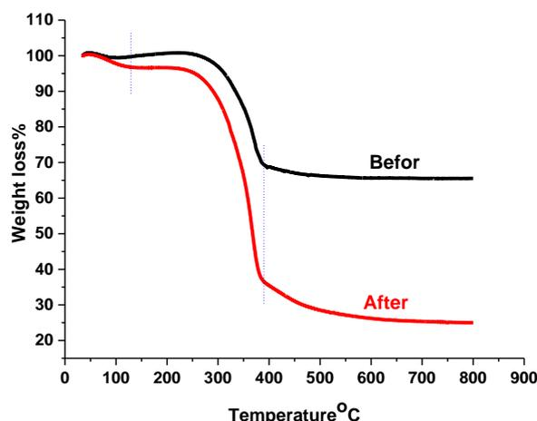
Fig.5:TGA of the experimental wood before and after heat treatment.
