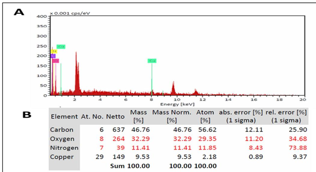
**Figure 5:** EDX micrographs of activated PET/C blended fabrics and loaded with biosynthesized CuO-NPs\*(1000x). (B) PET/C+E+CuO. \*After five washing cycles according to AATCC Test Method (61-1989). E=Cellulases
