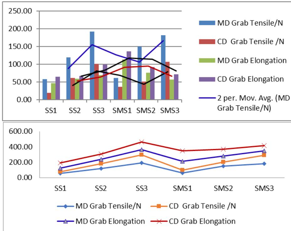
Fig. 8. Graphs Tensile & Elongation Test Results and Variable Relationships
