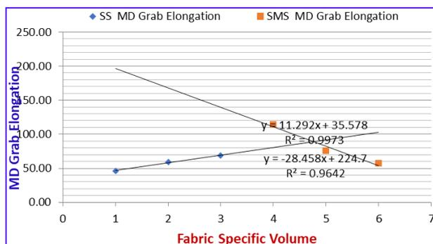
Fig. 14. Shows Correlation Coefficient and Regression between Fabric Specific Volume and MD Elongation Test Results.
