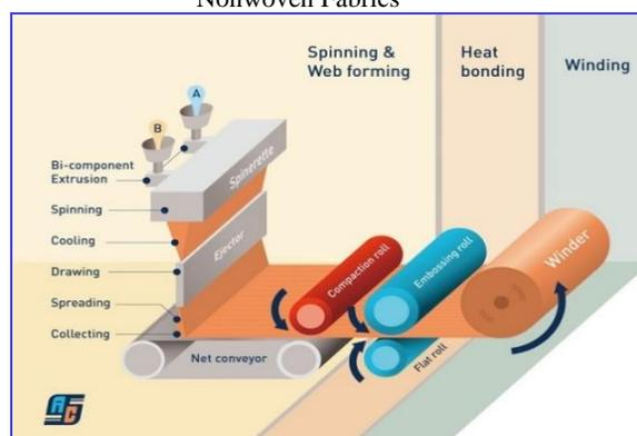
Fig.5. Polypropylene Spun Bond Nonwoven Fabric
