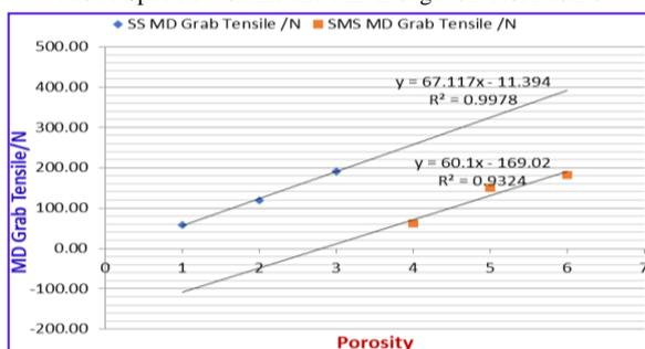
Fig. 16. Shows Correlation Coefficient and Regression between Fabric Porosity % and MD Grab Tensile
