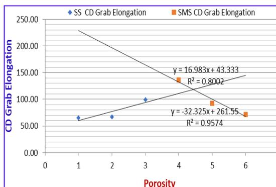
Fig. 19. Shows Correlation Coefficient and Regression between Fabric Porosity % and CD Grab Tensile
