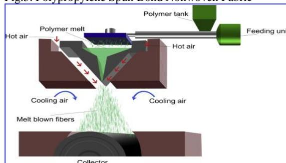
Fig. 6. B Spun-bonding melt-blowing
