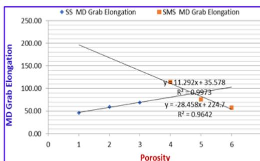
Fig. 18. Shows Correlation Coefficient and Regression between Fabric Porosity % and MD Grab Tensile
