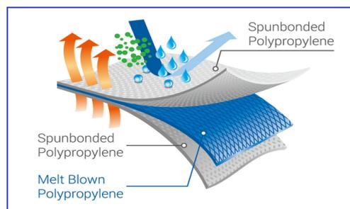
Fig. 2. (SMS) Spun bond Melt-blow Three Layers
