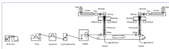
Fig. 3. Line of Manufacturing SS Polypropylene Nonwoven Fabrics
