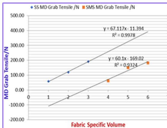
Fig. 12. Shows Correlation Coefficient and Regression between Fabric Specific Volume and MD Grab Tensile
