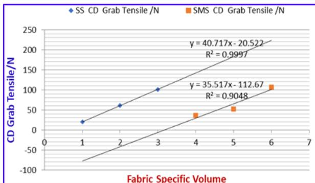
Fig. 13. Shows Correlation Coefficient and Regression between Fabric Specific Volume and CD Grab Tensile
