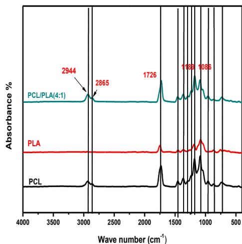
**Figure 2:** A comparative FTIR spectra for electrospun PCL, PLA and PCL/PLA (4:1) nanofiber scaffolds.
