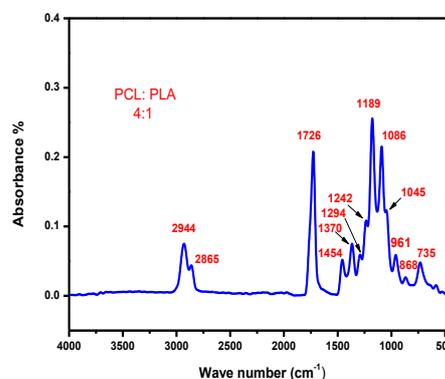
**Figure 1:** FTIR spectra of the electrospun PCL/PLA (4:1) copolymer Nano fiber scaffold.
