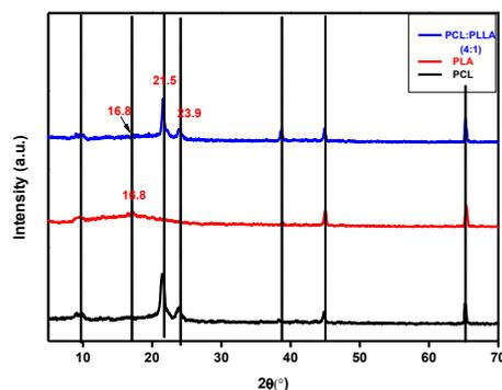
**Figure 3:** Comparative XRD pattern for the electrospun PCL, PLA and PCL/PLA (4:1) nanofiber scaffolds.
