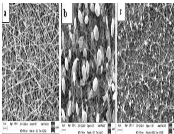
**Figure 4:** SEM images for electrospun PCL, PLA, and PCL/PLA copolymer nanofiber scaffolds, respectively.
