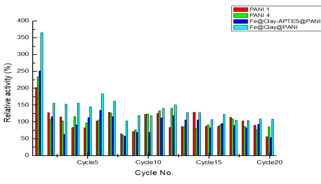
Fig. 3. Reusability of immobilized  $\beta$ -glucosidase on different carriers (with glutaraldehyde treatment), (PAN1) nano-polyaniline fibers No. 1, and (PAN4) nano-polyaniline fibers No. 4., Fe@Clay-APTES@PANI, and Fe@Clay@PANI
