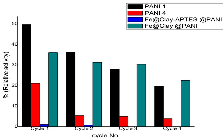
Fig. 5. Reusability of immobilized CMCase on different carriers (with glutaraldehyde treatment), (PAN1) nano-polyaniline fibers No. 1, and (PAN4) nano-polyaniline fibers No. 4., Fe@Clay-APTES@PANI, and Fe@Clay@PANI.
