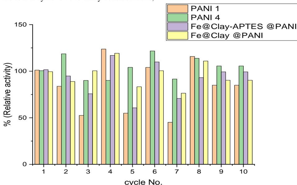
Fig. 4. Reusability of immobilized FTase on different carriers (with glutaraldehyde treatment), (PANI1) nano-polyaniline fibers No. 1, and (PAN4) nano-polyaniline fibers No. 4., Fe@Clay-APTES@PANI, and Fe@Clay@PANI.
