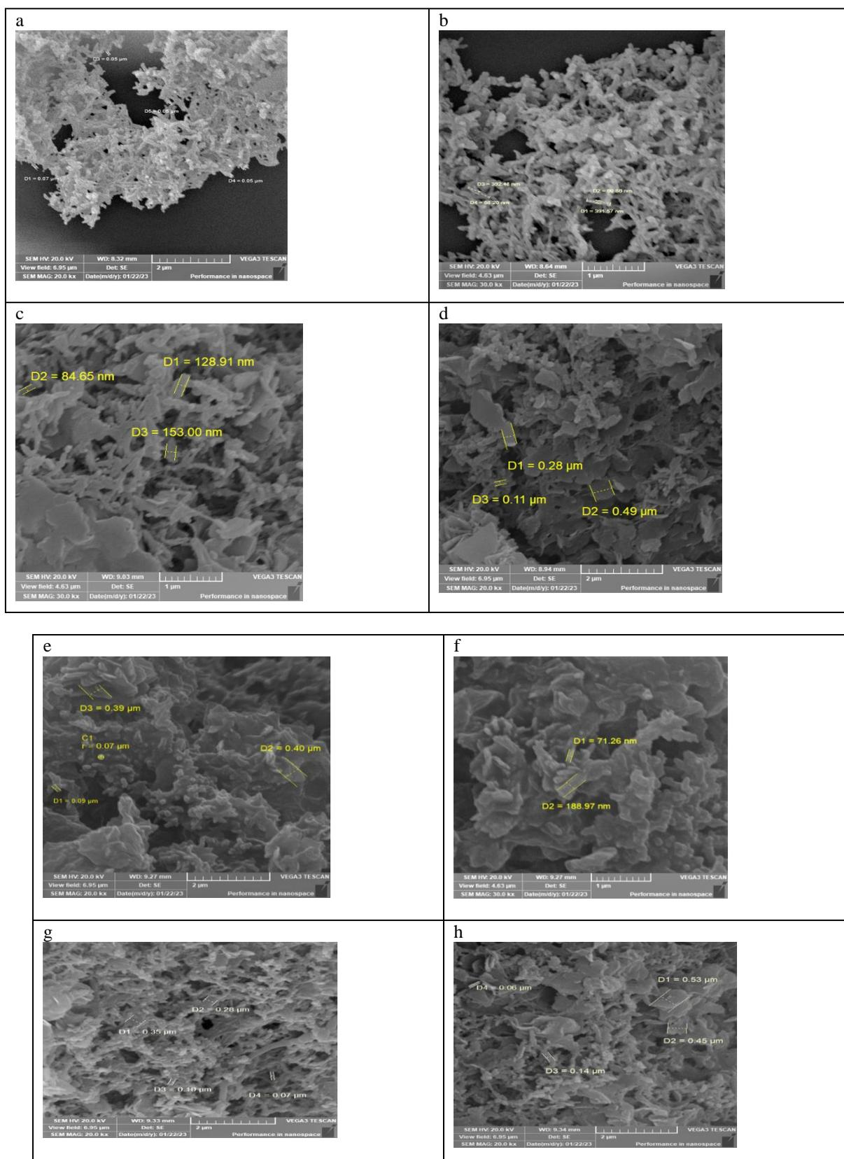
Fig. 1. SEM images of PANI (a, and b), Fe@Clay@PANI (c, and d), PANI Fe@Clay-FTase (e, and f), and PANI Fe@Clay- $\beta$ -Glu (g, and h).
