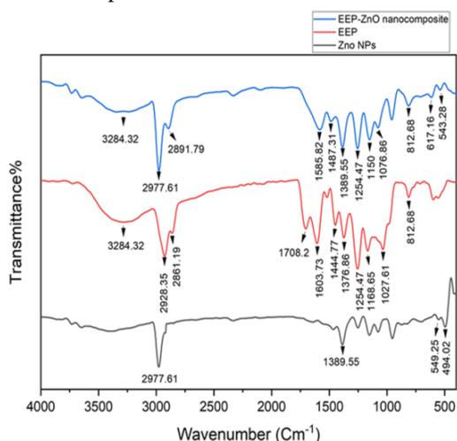
Fig. 3: FT-IR spectrum of ZnO NPs, propolis extract (EEP) and EEP-ZnO nanocomposite.
