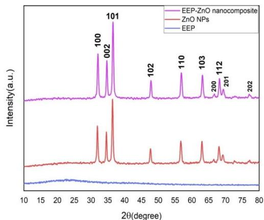
**Fig. 1:** XRD patterns of EEP, ZnO NPs and EEP-ZnO nanocomposite.
