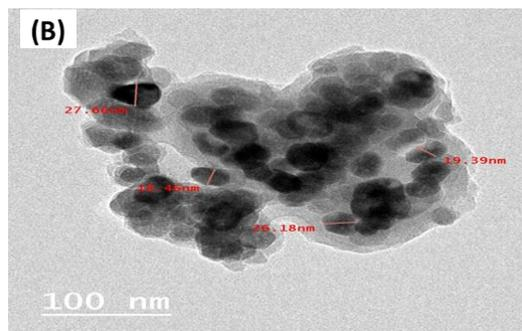
**Fig. 2:** HR-TEM of (A) ZnO NPs and (B) EEP-ZnO nanocomposite.
