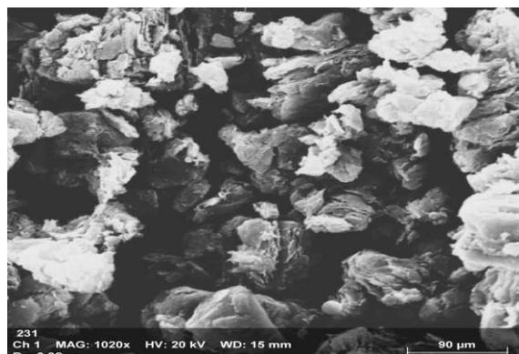
**Figure 10.** The particle size of synthesized graphene
