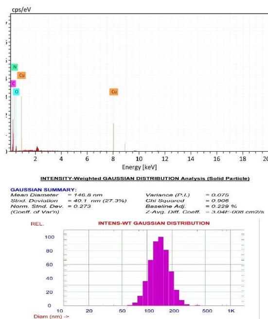
**Figure 14.** Molecular distribution of the synthesized copper nanoparticles
