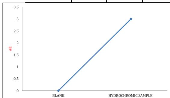
**Figure 3.** Total color differences “ $\Delta E$ ” between blank and wet hydro-chromic sample–
