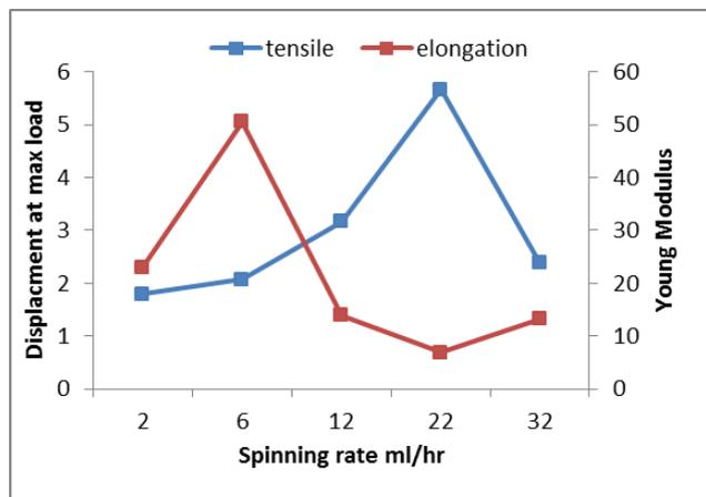
**Figure 4:** Mechanical Properties of Electro spun cellulose acetate fibers.
