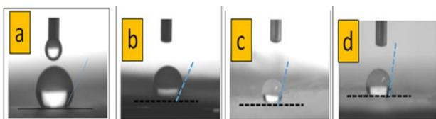
**Figure 3:** Contact angles of Cellulose acetate with different speeds; Where: a) 6 ml/hr, b) 12 ml/hr, c) 22 ml/hr and d) 32 ml/hr.
