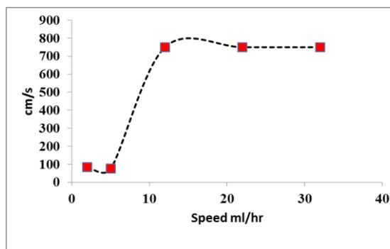
**Figure 5:** Air permeability of the prepared cellulose acetate Nano fibers
