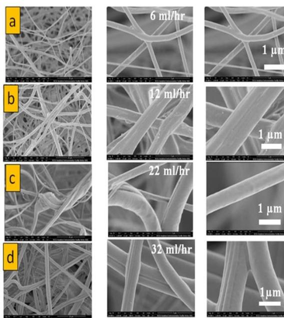
**Figure 2:** Scanning Electron Microscope of Cellulose acetate with different speeds. Where :a) 6 ml/hr, b) 12 ml/hr, c) 22 ml/hr and d) 32 ml/hr.
