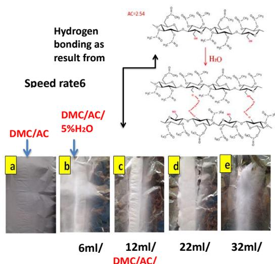
**Figure 1:** Optical images for produced Electrospun fibers using binary and ternary solvent at different speed rate.
