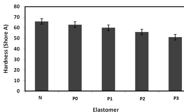
**Figure 6.** Hardness (Shore A) of vulcanized N, P0 and P1, P2 & P3 elastomer blends.
