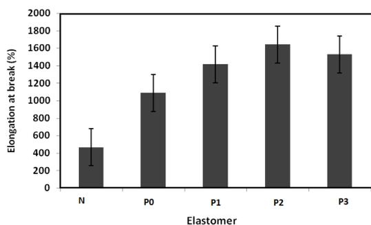
**Figure 4.** Elongation at break (%) of vulcanized N, P0 and P1, P2 & P3 elastomer blends.
