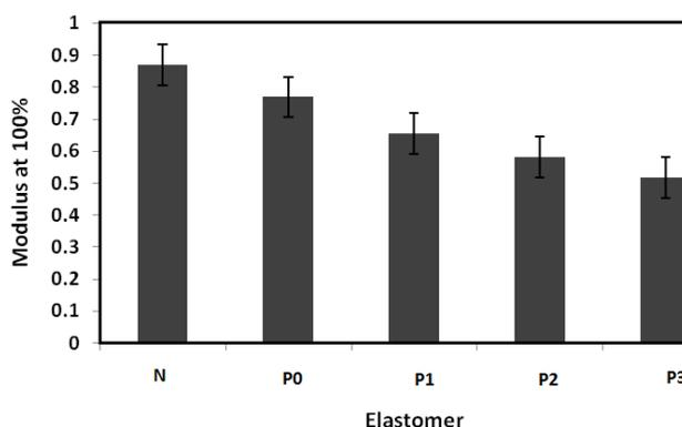
**Figure 5.** Modulus at 100% elongation of vulcanized N, P0 and P1, P2 & P3 elastomer blends.
