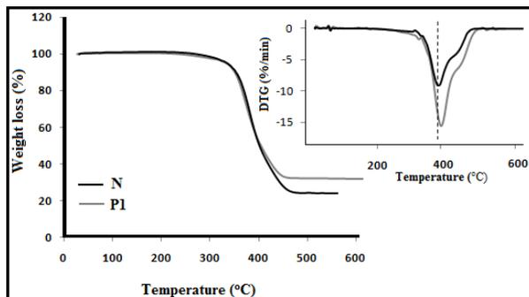
**Figure 8.** TGA and DTG of P1 and N elastomers
