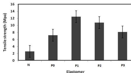
**Figure 3.** Tensile strength of vulcanized N, P0 and P1, P2 & P3 elastomer blends.
