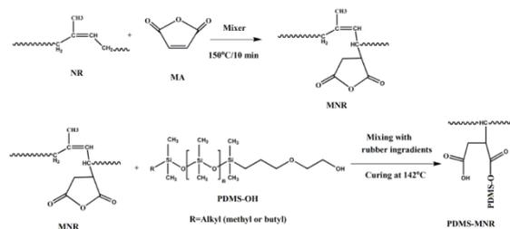
**Scheme 1.** The possible reaction mechanism of MNR with PDMS-OH to obtain MNR-PDMS elastomer blend.
