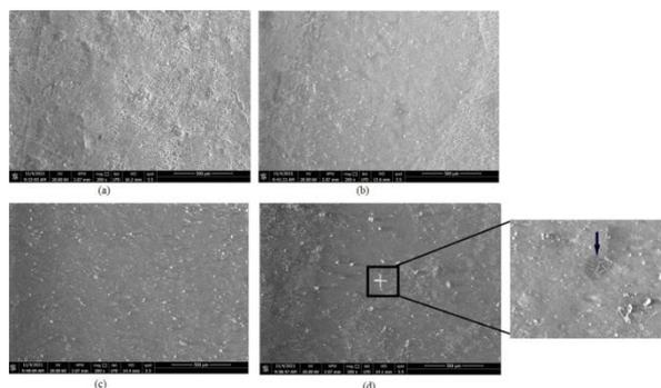
**Figure 7.** SEM micrographs of vulcanized (a) N, (b) P0, (c) P1 and (d) P2 elastomers.
